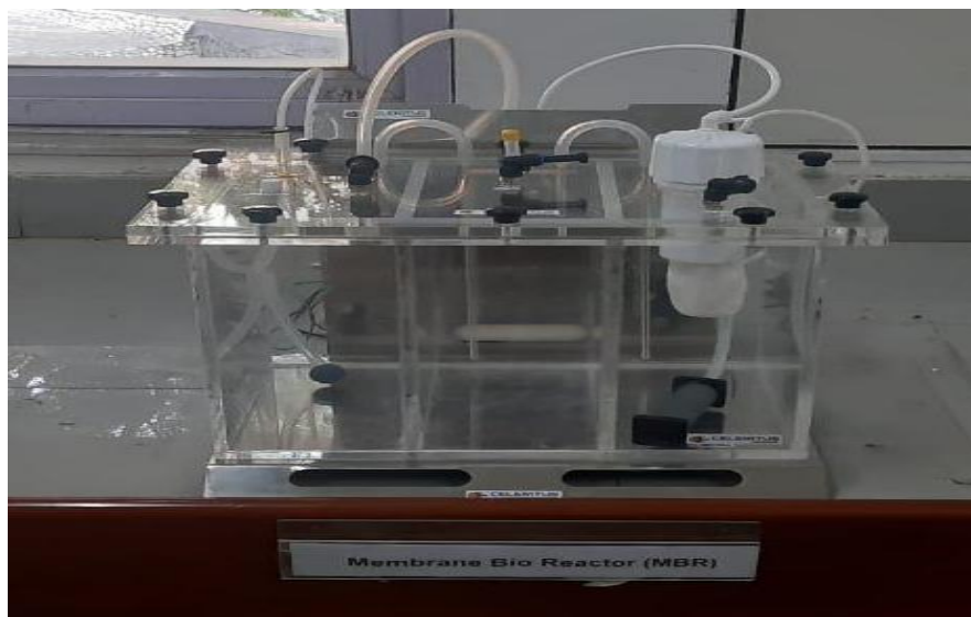
Fig. 3.1. Laboratory scale submerged membrane bioreactor
