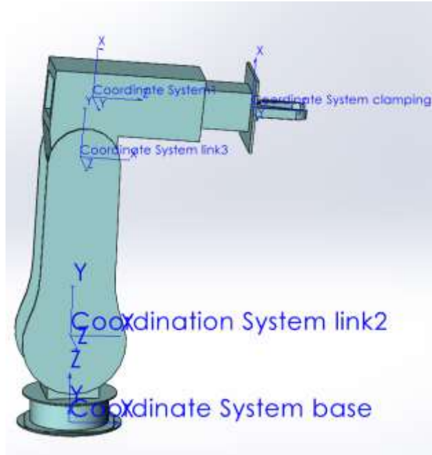
Figure-3.7 Assembly of the manipulator
