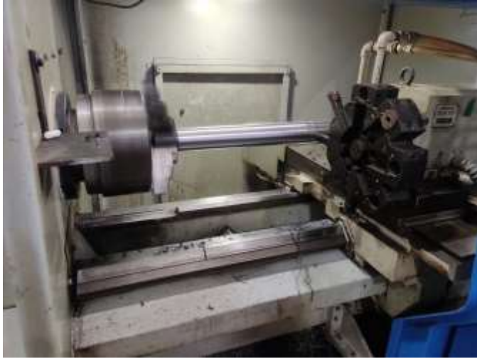
Figure 7 HMT CNC Turning lathe, CNC tool and Insert
