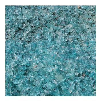
Cullet is crushed glass that has a similar composition to the mineral mixture and is derived from regrind from earlier production runs and recycling sources. A glass batch may consist of 25 to 60 percent cullet by volume. It is included because its ability to melt in the furnace before the other minerals aids in the batch's transformation into molten glass. It's an essential energy-saving component that helps minimise greenhouse gas emissions by lowering the amount of
