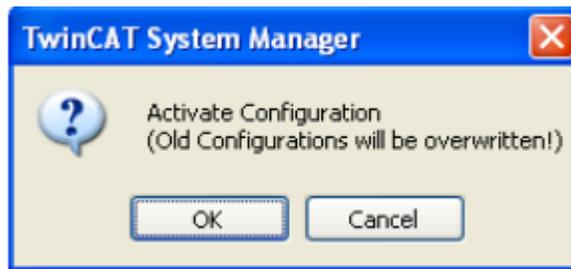
3. Select OK to Restart TwinCAT system in Run mode
