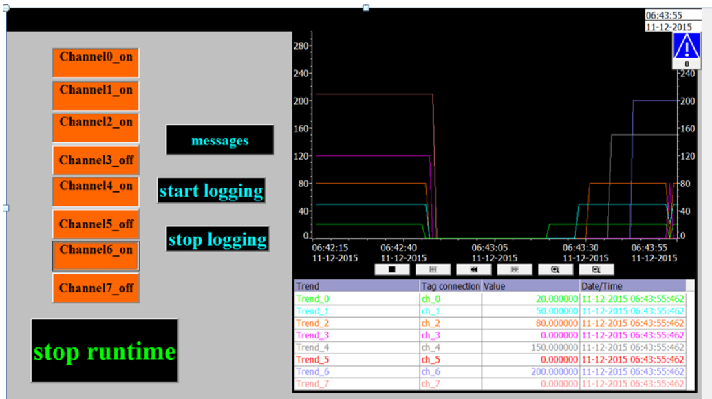
Figure 5.11: HMI SCREEN for multichannel interfacing
