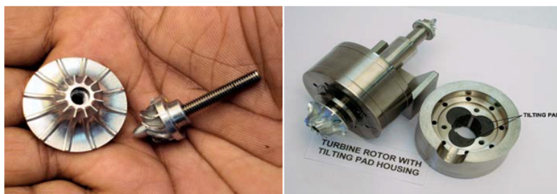
Figure 2.7: Miniature turbomachinery: expansion turbine and brake wheel
