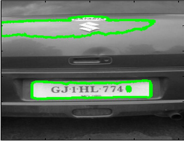
Fig. 6 Result of localization by thesholding
