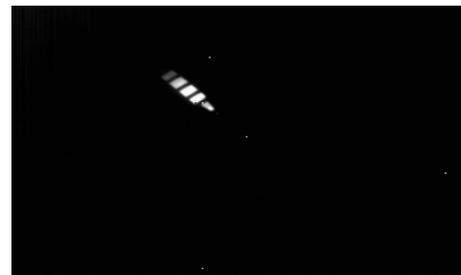
Fig. 10. Image (one of the frames of an AVI file) of a Soldering Iron taken by the IR Camera
