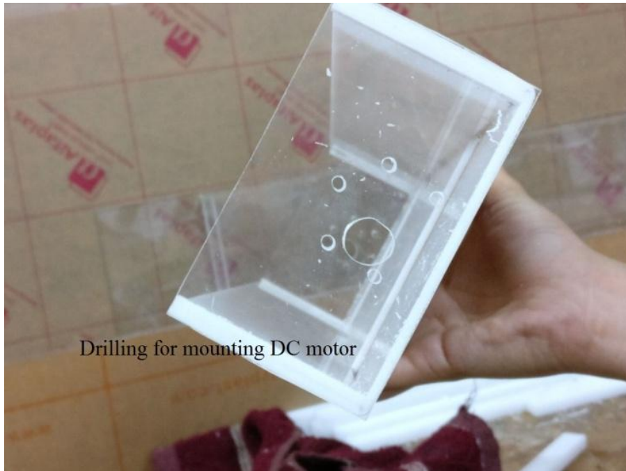
Figure 3 Holes for mounting the dc motors
