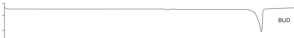
Figure 12. Literature DSC spectrum of pure budesonide with a reported melting point of 261.58°C (Sahib et al., 2011).
