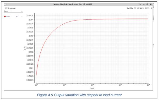
Load regulation in an operational amplifier (op-amp) refers to its ability to maintain a stable output voltage when subjected to changes in the load resistance connected to its output. Load regulation is an important characteristic to consider, as it affects the op-amp's ability to provide a consistent output voltage regardless of variations in the load.
