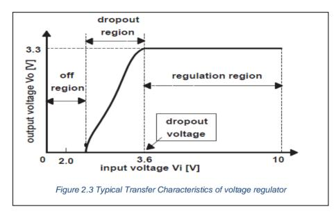
Figure 2.3 illustrates the typical transfer characteristic curve of a voltage regulator, which is divided into three main regions: the OFF region, the dropout region, and the regulation region.
