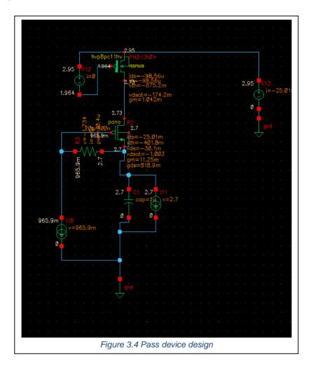
Designing a Pass Device is the first fundamental stage of LDO design. Therefore, the Pass device design is represented in the diagram below together with several other significant devices. These devices are in place because they in some way aid in the proper operation of the pass device.
