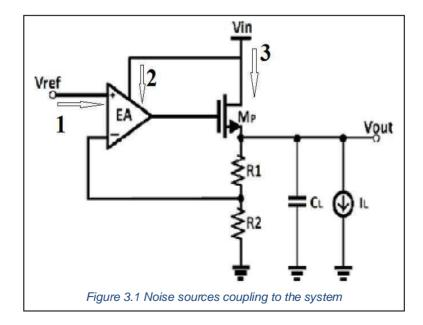
Among the sources of supply noise entering the system depicted in fig 3.1, the noise from voltage reference circuit is minimal comparatively from sources 2 and 3. This may be from the fact that usually the output of the reference circuit is filtered out to reduce the ripples in the output.
