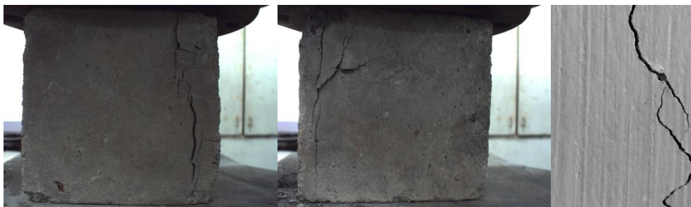
Figure 54. Testing images of cracks for line emphasis method.
