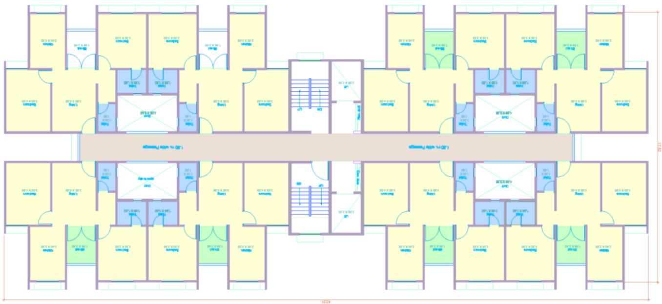
Figure 33 : 2 BHK Block Layout Plan
