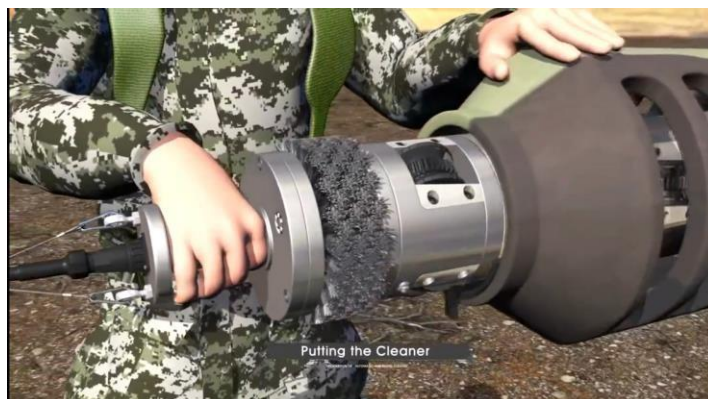
Figure 3. 6 putting SPM inside barrel
