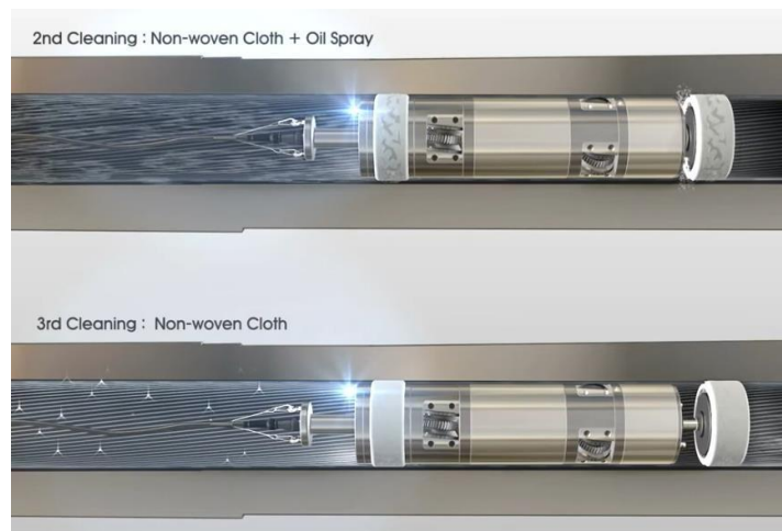
Figure 3. 8 stepwise cleaning process of SPM
