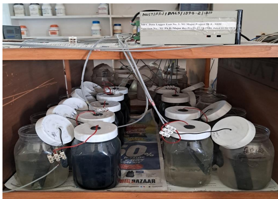
Figure 4: Batch mode MFC systems containing different SB concentrations such as 5 mM, 10 mM, 15 mM and 20
