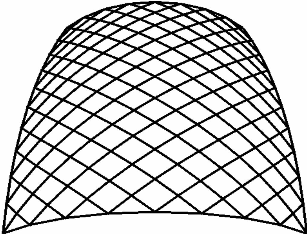
Figure 5.20 Ellipsoidal lamella barrel vault
