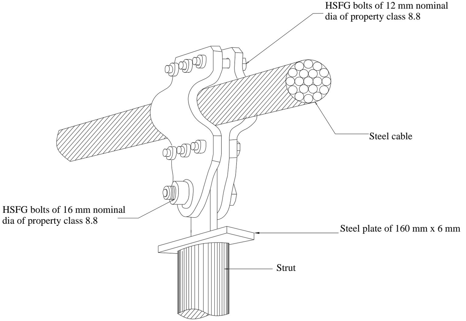
Figure 4.8 Cable strut connection
