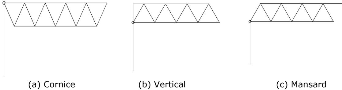
Figure 5.12 Different types of grid edge profile
