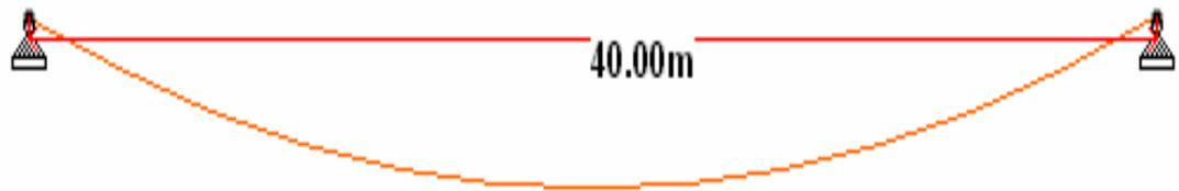
Figure 3.19- Beam made of only one element
