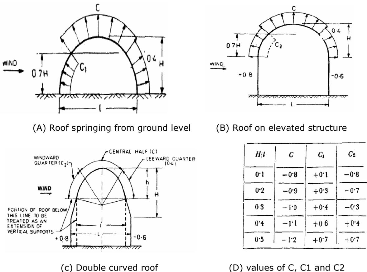
Figure 2.12 External pressure coefficients for curved roof as per
