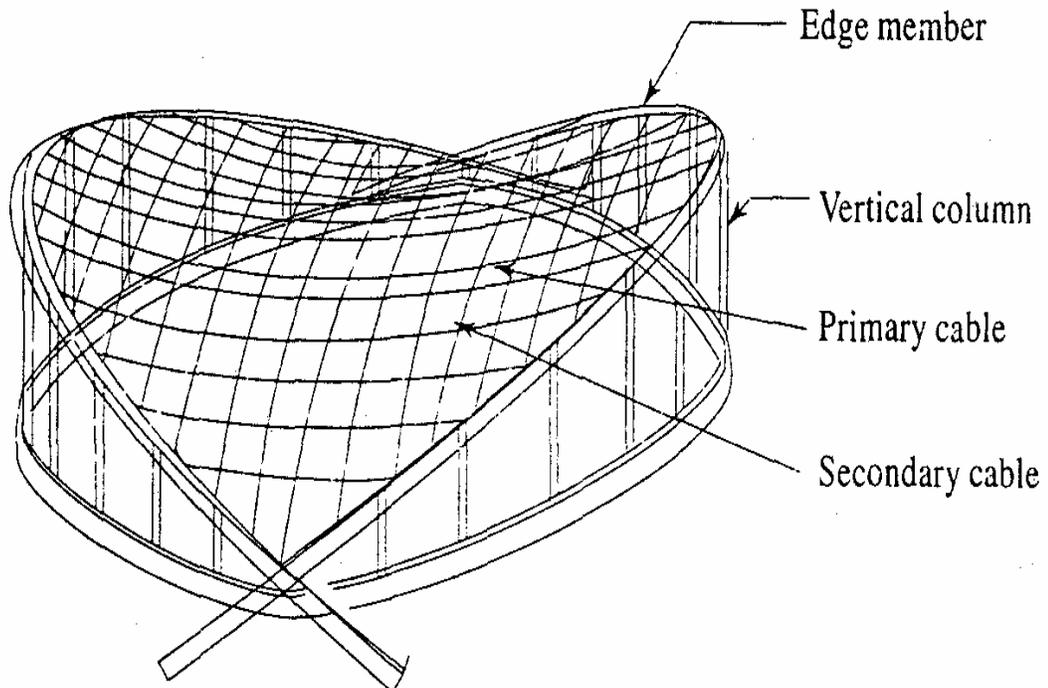
Figure-3.15 Anticlastic cable for circular buildings
