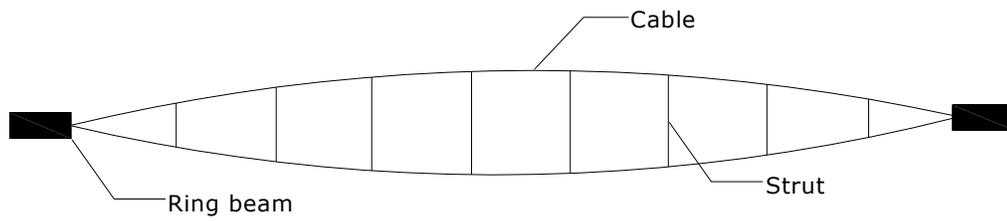
Figure-3.10 Double layer cable-convex shape for circular buildings
