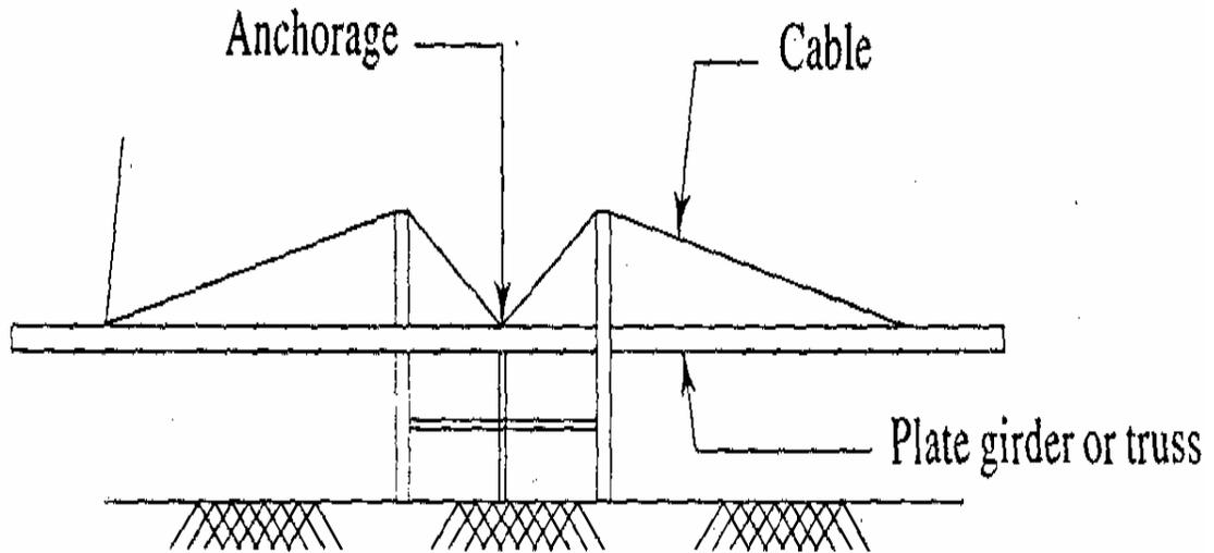
Figure 3.2- Cable supported roof system
