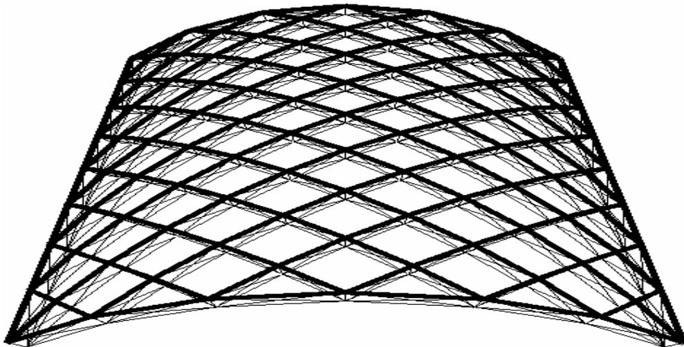
Figure 5.18 Lamella (diagonal) truss barrel vault
