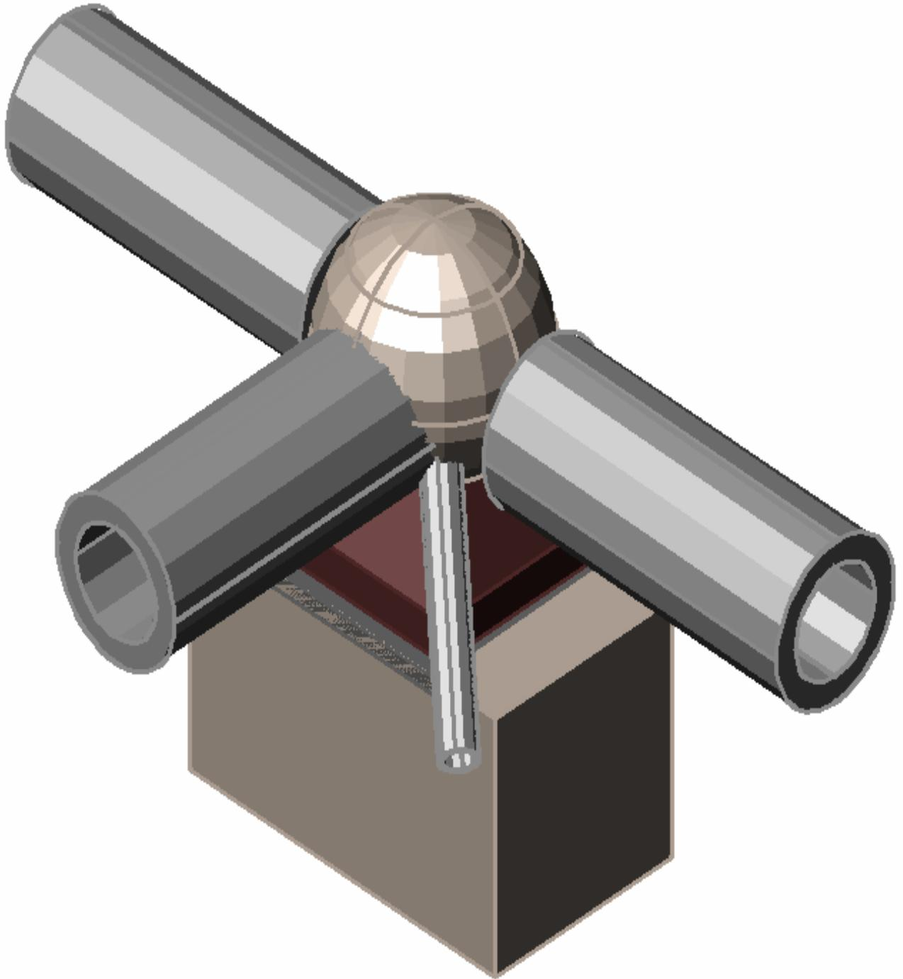
Figure 6.8 3d view of steel tube to concrete column
