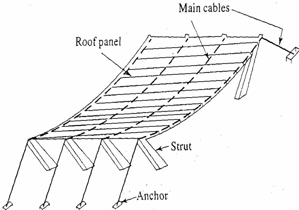
Figure-3.5 Singly curved single layer cable suspended roof
