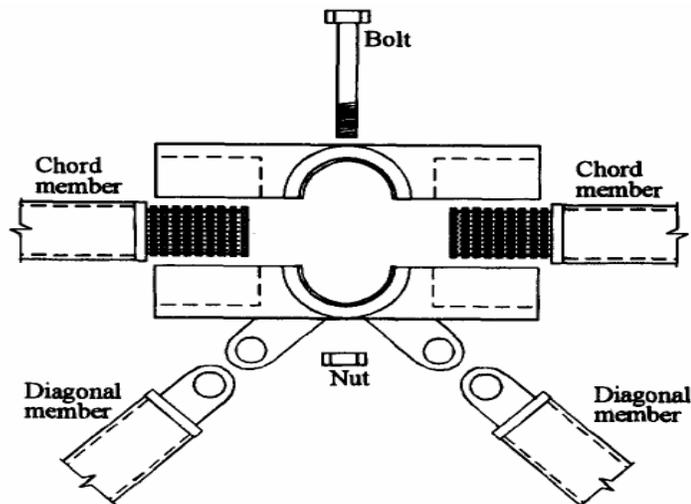
Figure 2.11 Typical Nodus node with member end fittings
