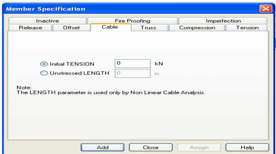
Figure 2.14 Application of initial tension
