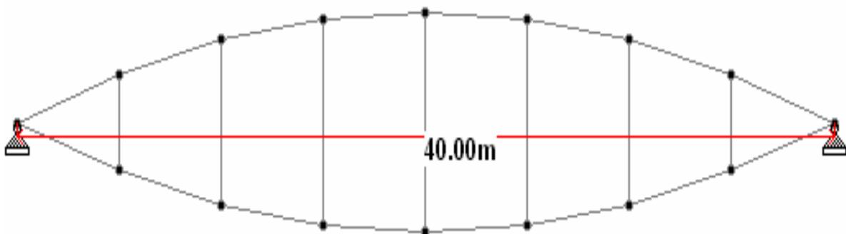
Figure 3.21- Double curved cable structure
