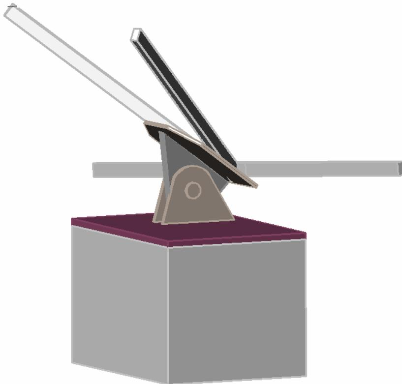
Figure 6.20 3d views of connection of RHS section to concrete column
