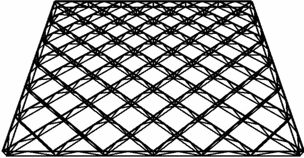
Figure 5.10 Diagonal trusses ---double layer grid
