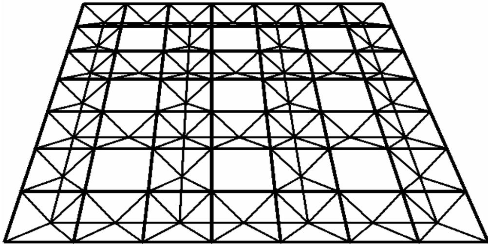
Figure 5.8 Reduced two way on two way ---double layer grid
