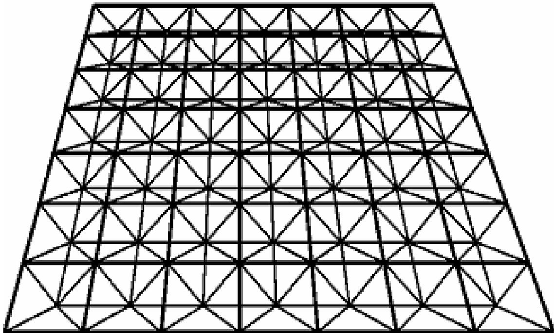
Figure 5.5 Two-way on two-way (square on square offset)
