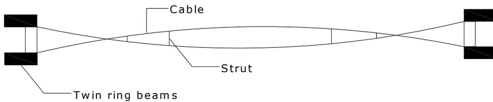
Figure-3.12 Double layer cable-intermediate shape for circular buildings
