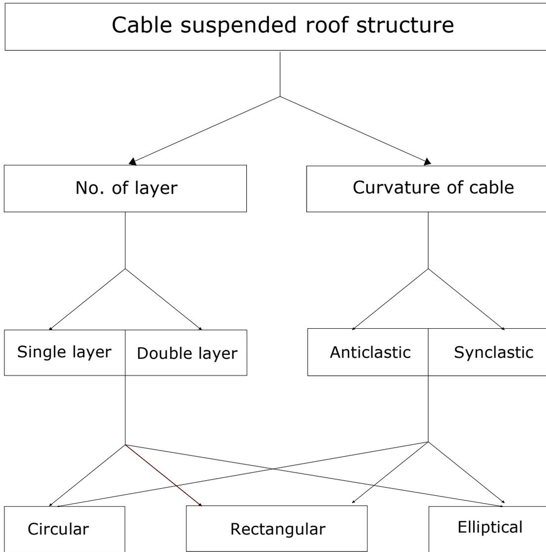
Figure 3.4- Classification of cable suspended structures
