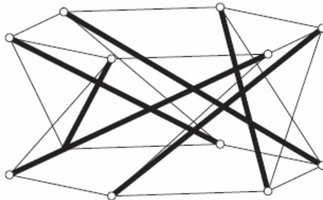
Figure 1.8 Tensegritic structure modules
