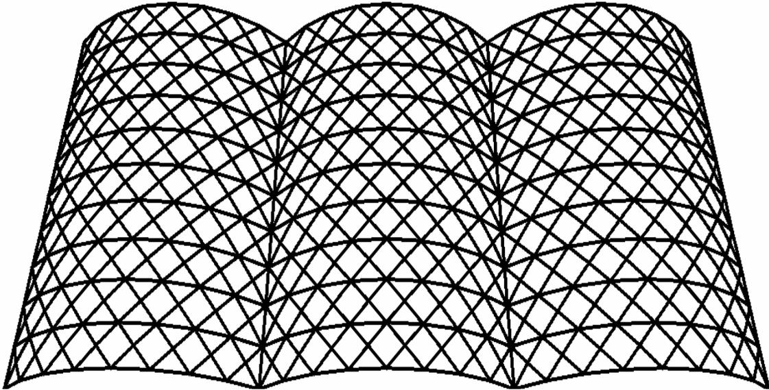
Figure 5.21-Compound three way barrel vault
