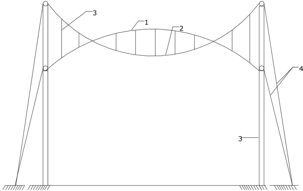
Figure-3.9 Double layer cable-concave-convex combination shape for rectangular buildings
