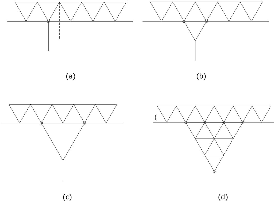
Figure 5.11- Different methods of supporting the grid
