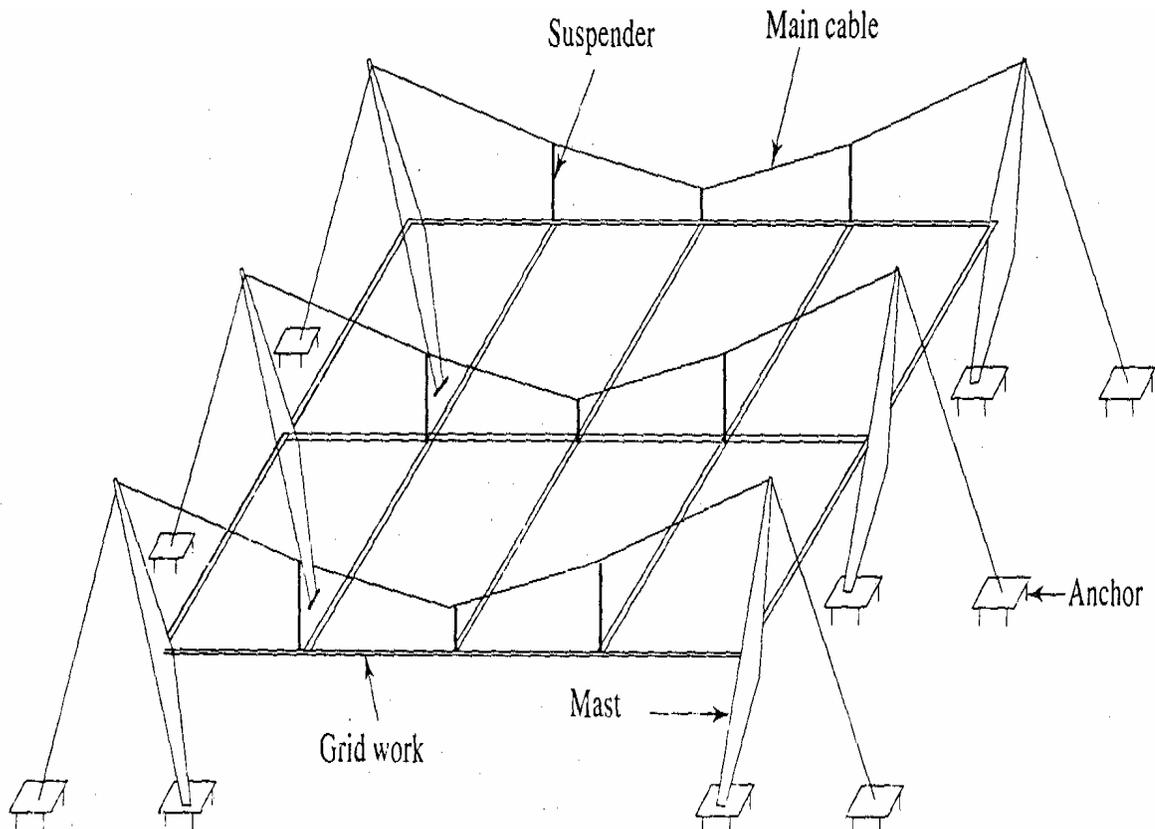
Figure 3.3- Cable suspended roof system
