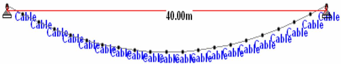
Figure 3.20- Cable made of small straight elements
