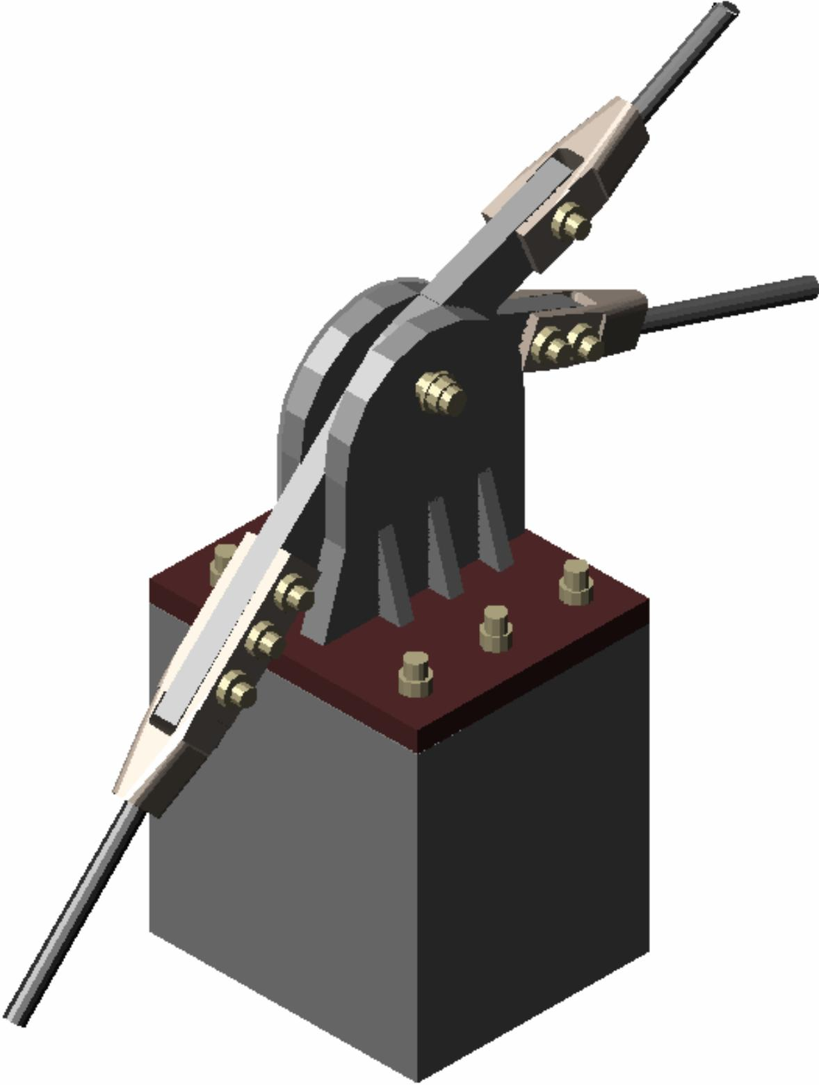
Figure 4.11 3d view of cable-column connection
