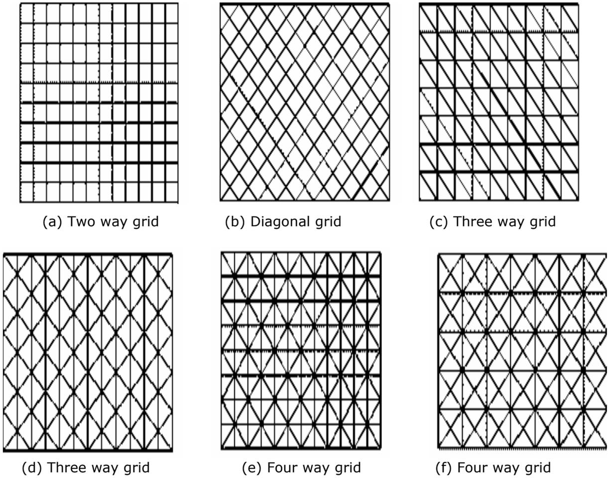
Figure 5.3 Different types of single layer grid
