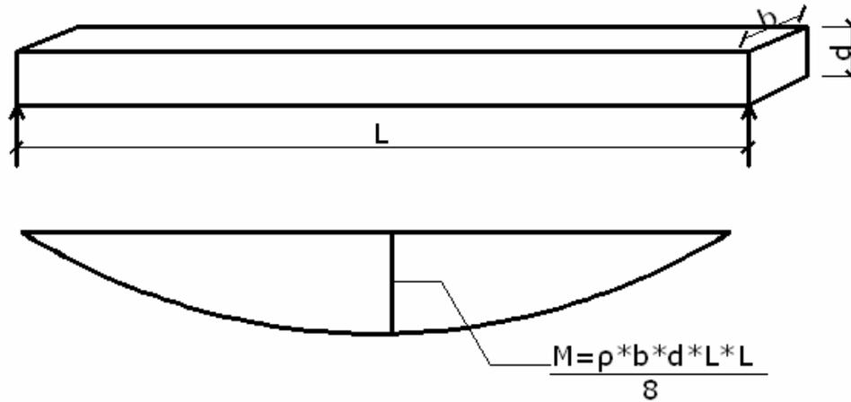
Figure 1.1 Bending in rectangular beam
