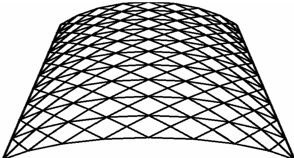
Figure 5.16 Three way barrel vault
