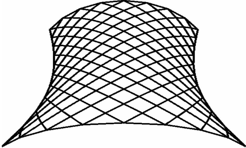
Figure 5.19 Hyperboloid lamella barrel vault
