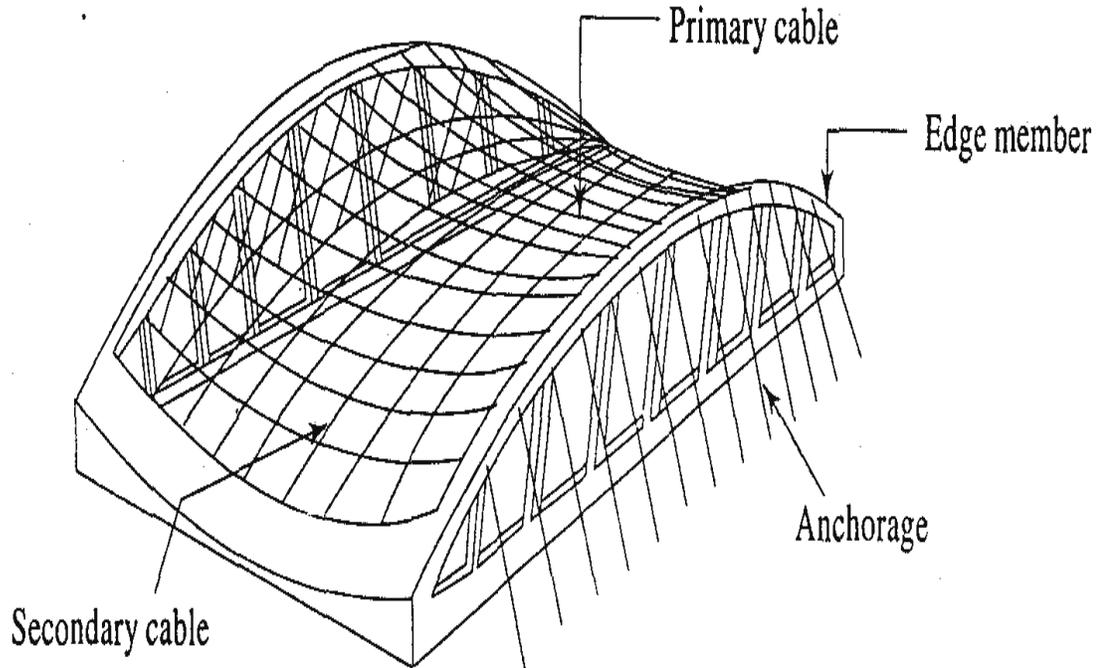
Figure-3.14 Anticlastic cable for rectangular buildings
