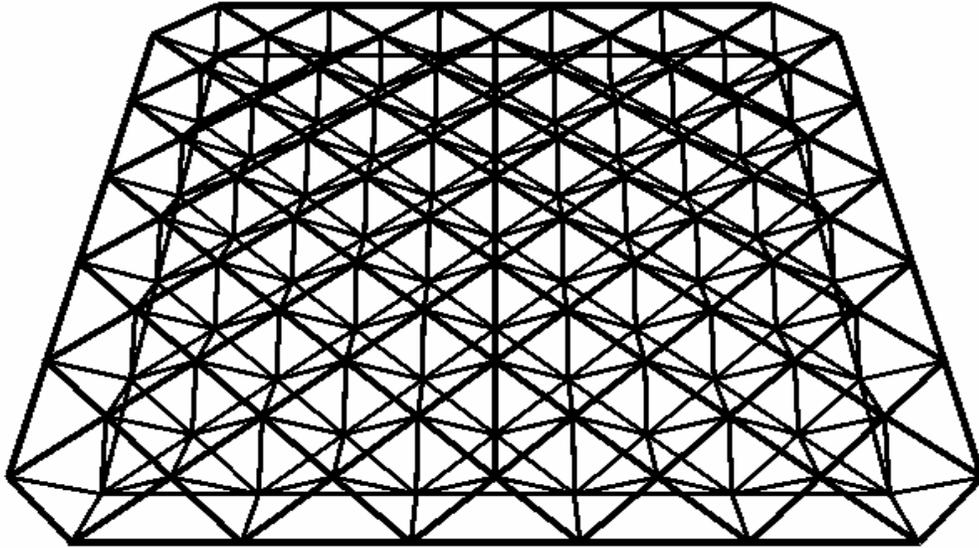
Figure 5.6 Diagonal on diagonal---double layer grid
