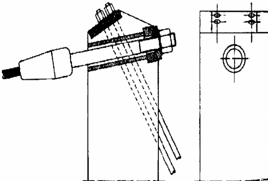
Figure 2.6 Attachment of cable with socket terminal to top of concrete column
