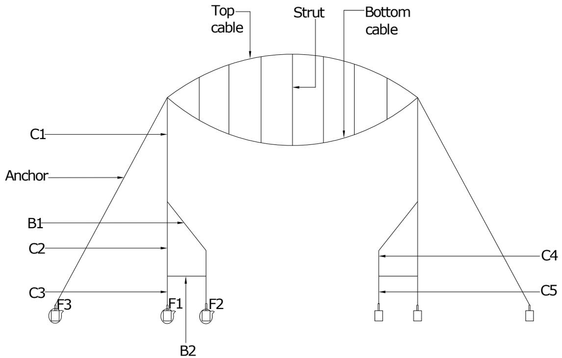
Figure 4.6 Identity of double layer cable structure
