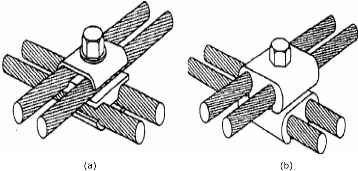
Figure 2.7 (a) Fit on site cable clamp connection
