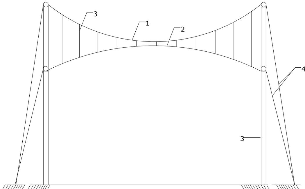
Figure-3.8 Double layer cable-concave shape for rectangular buildings
