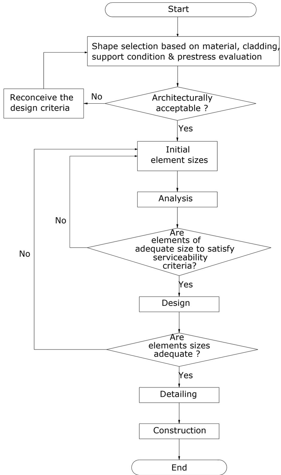
Figure 4.1 Flow chart for general design approach of cable structure
