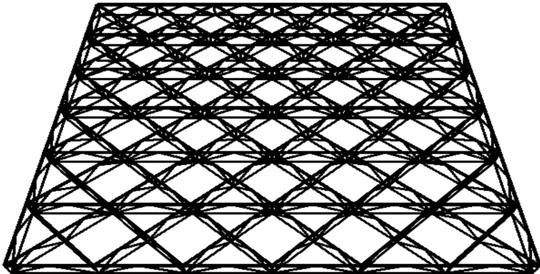
Figure 5.7 Three way truss grid---double layer grid
