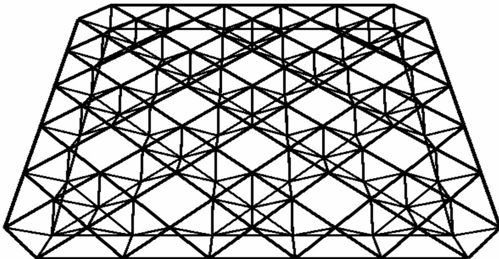
Figure 5.9- Reduced diagonal on diagonal ---double layer grid
