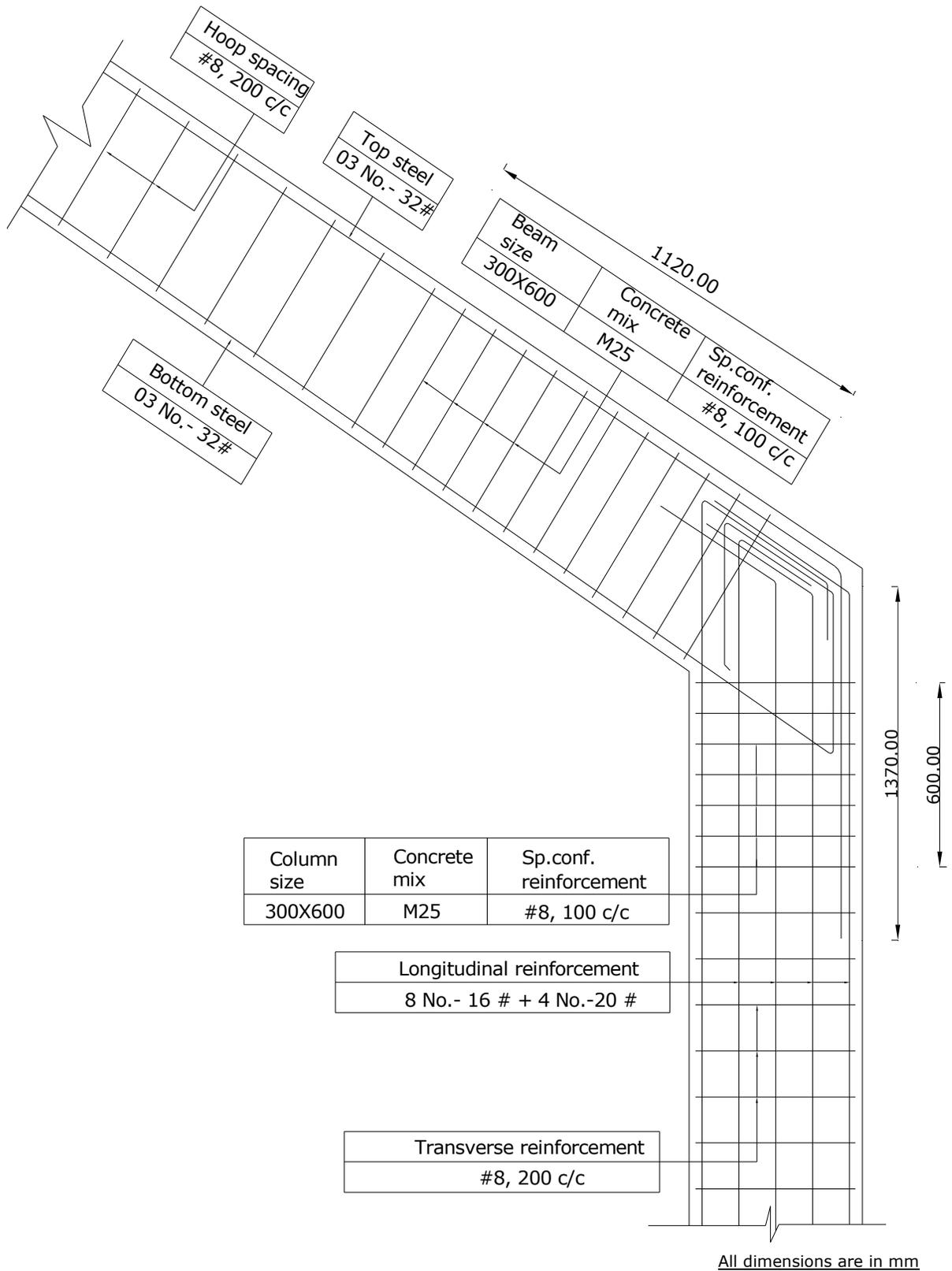
Figure 6.11 Beam-column junctions (Joint-B)
