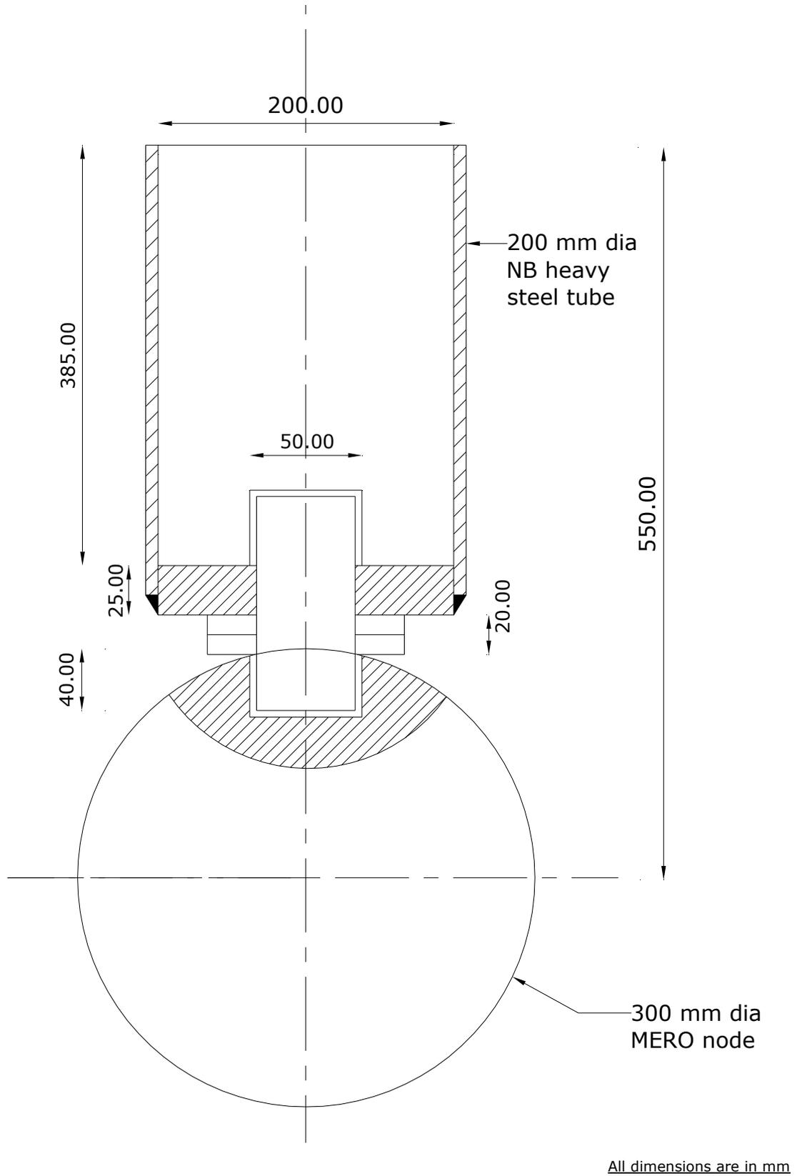
Figure 6.9 Typical stub details
