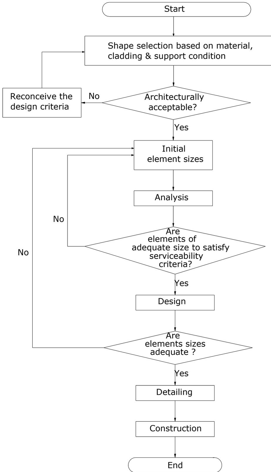
Figure- 6.1 Flow chart for general design approach of double layer grid and braced barrel vault structures
