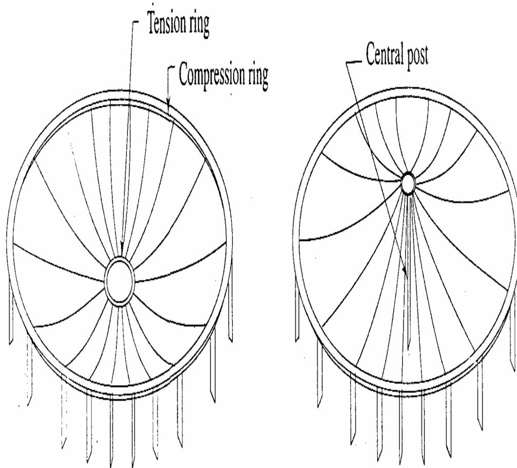
Figure-3.6 Doubly curved single layer cable suspended roof
