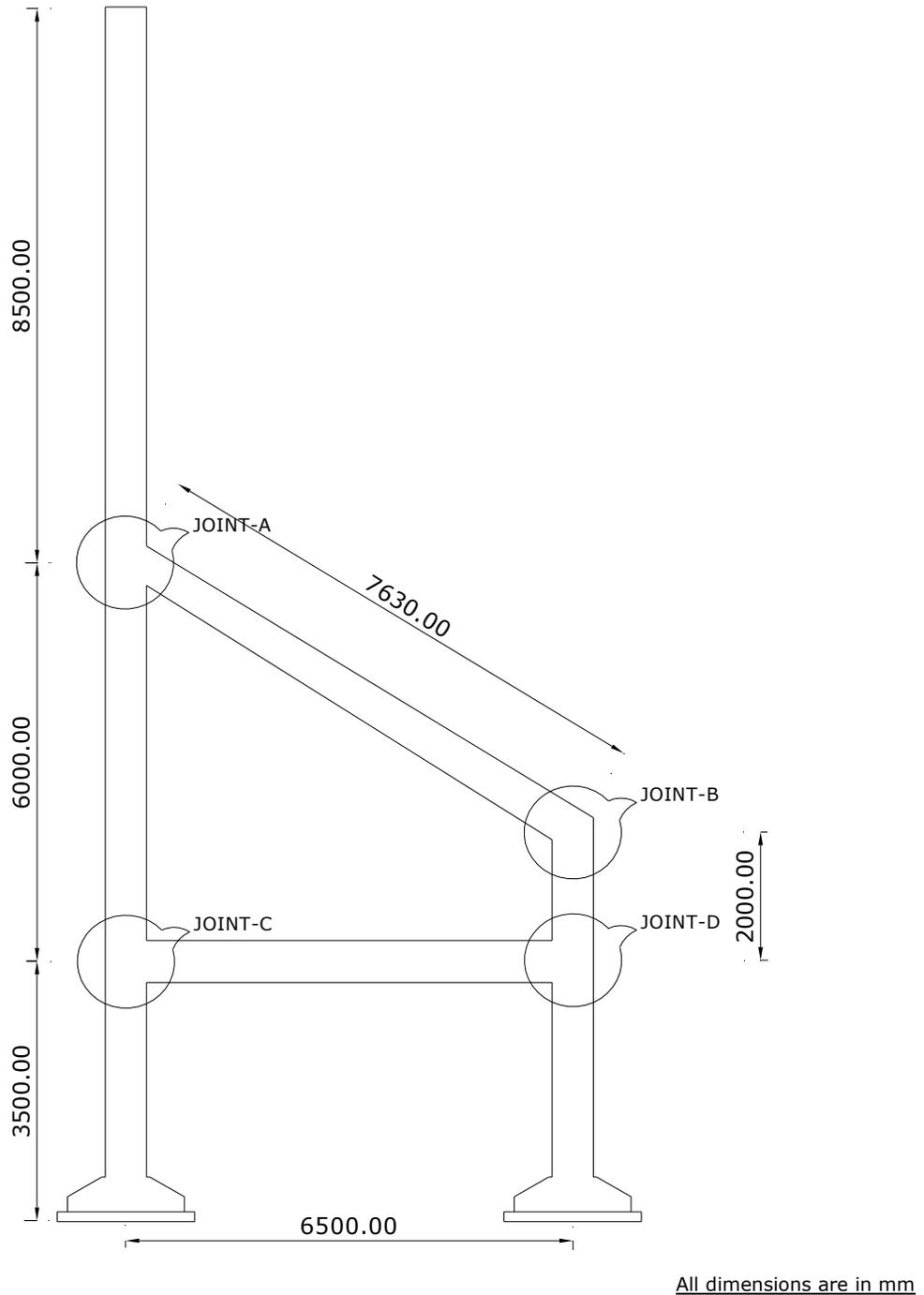
Figure 6.6 Supporting structural system modules for double layer grid
