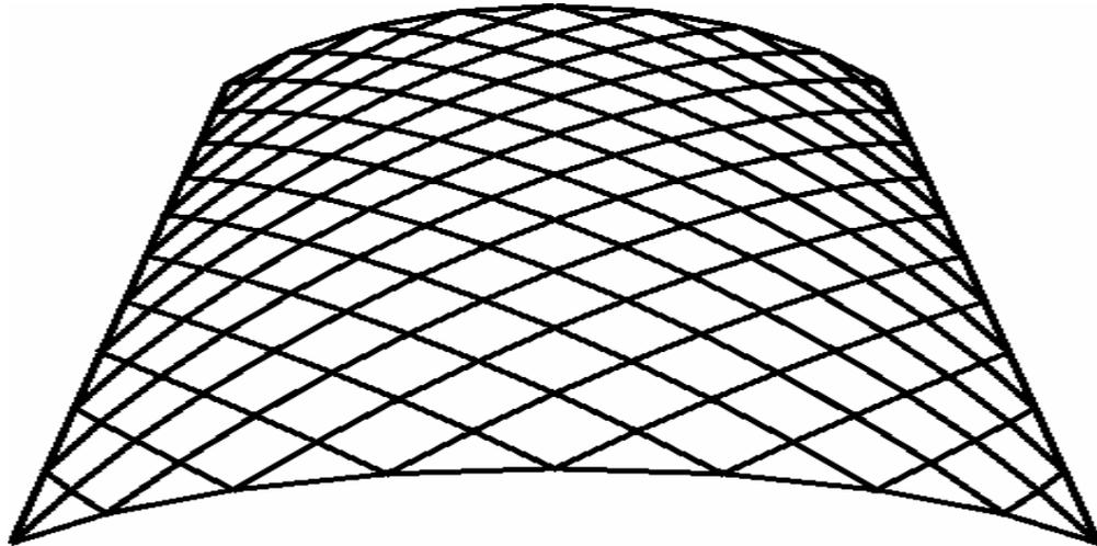
Figure 5.15 Lamella (diagonal) barrel vault
