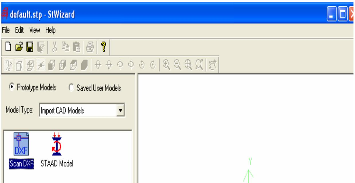
Figure 2.16 Import cad model in staad-pro
