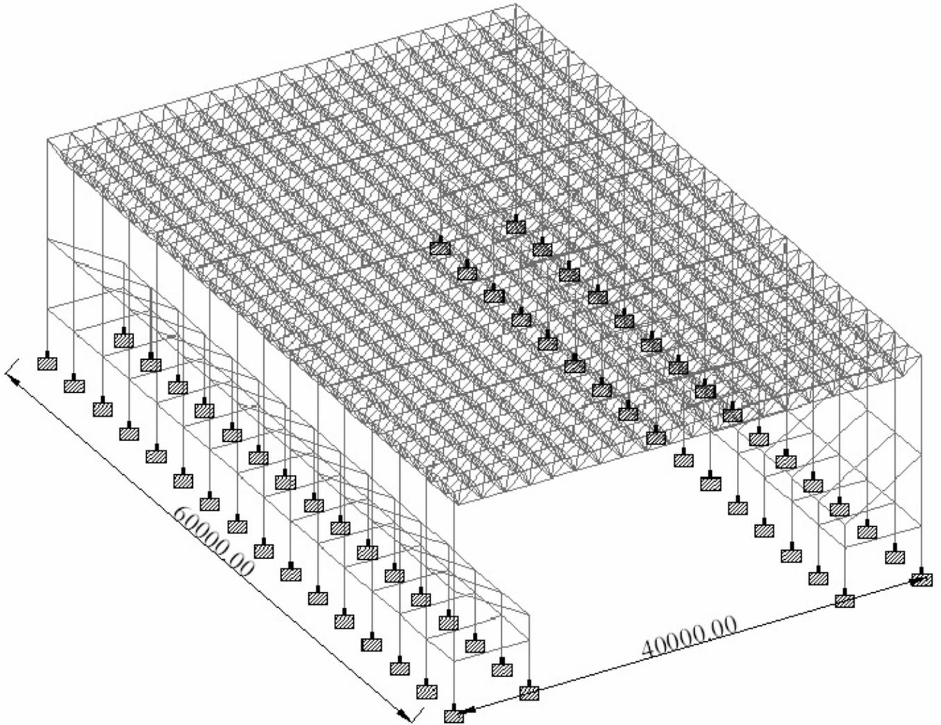
Figure 6.2 3d view of double layer grid
