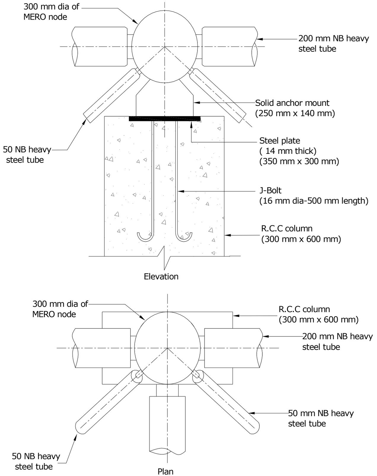
Figure 6.7 Detail of connection of steel tube to concrete column
