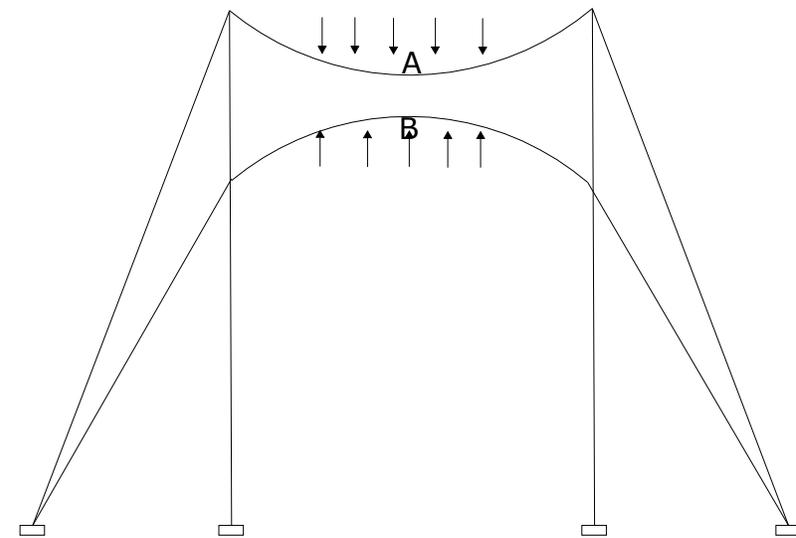
Figure-3.13 Structural behavior of a prestressed cable beam
