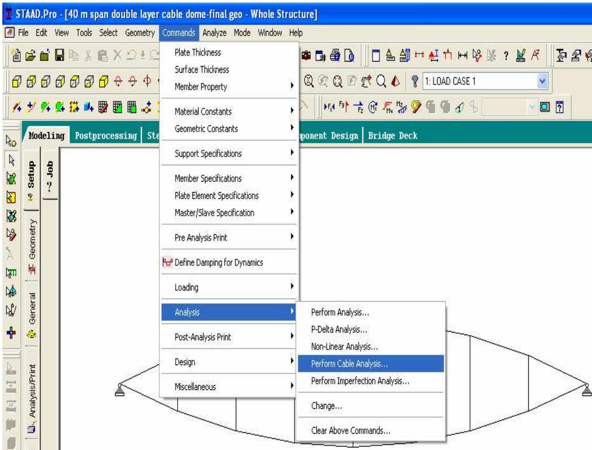
Figure 2.15 Performing cable analysis
