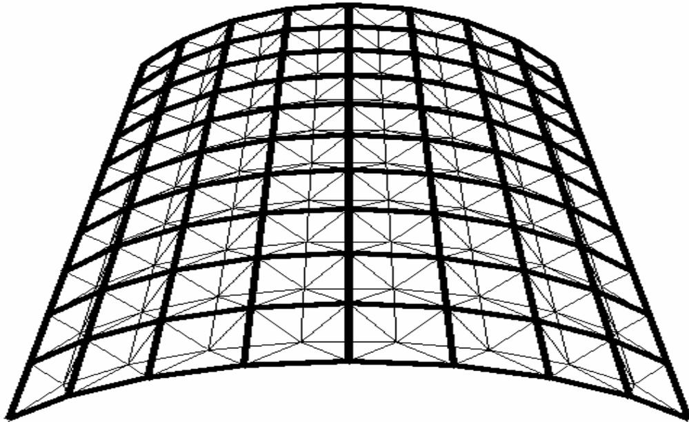
Figure 5.17 Two way on two way double layer barrel vault
