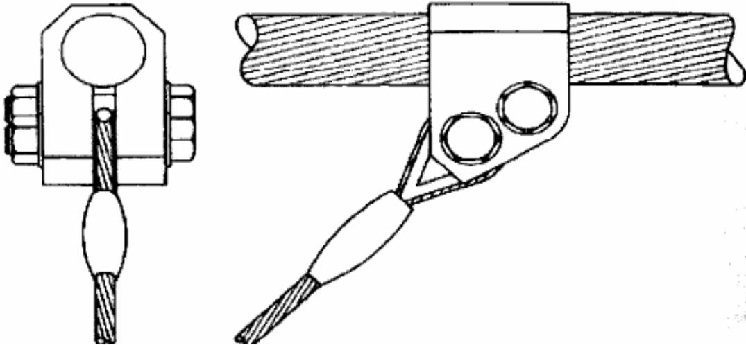
Figure 2.9 Detail showing clamp for connection of interior cable to edge cable
