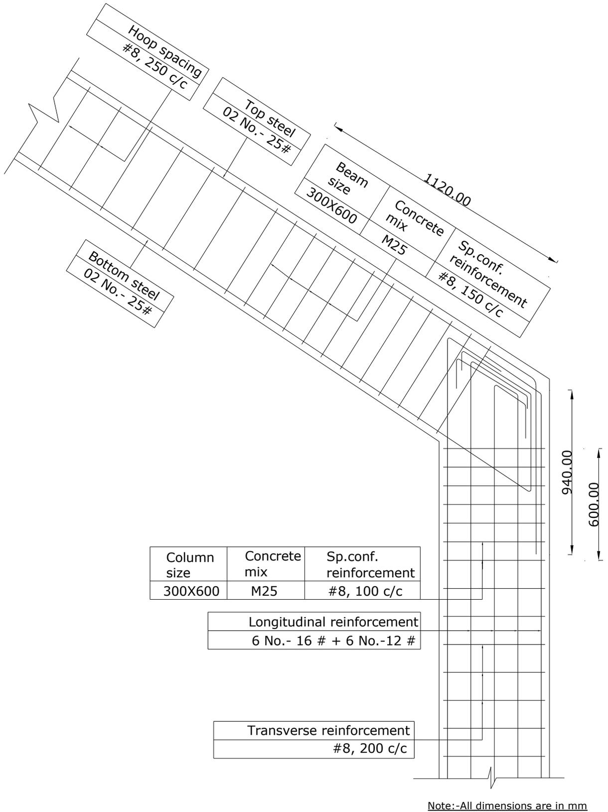
Figure 4.13 Beam-column junctions (Joint-B)
