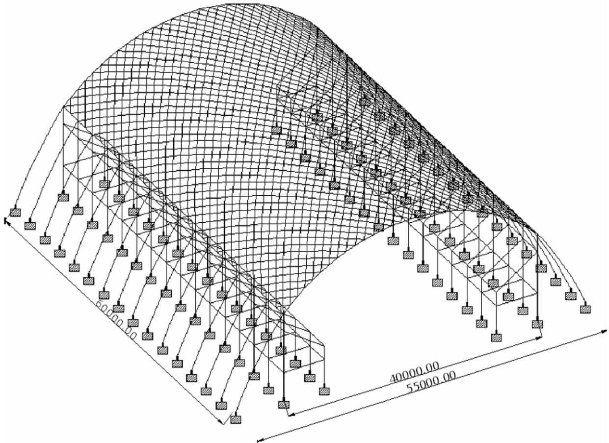
Figure 6.14 3d view of braced barrel vault
