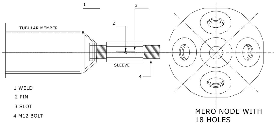
Figure 2.10 Typical Mero node and tubular member with its end fittings
