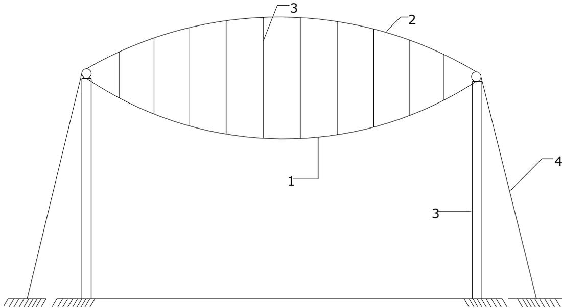
Figure-3.7 Double layer cable-convex shape for rectangular buildings
