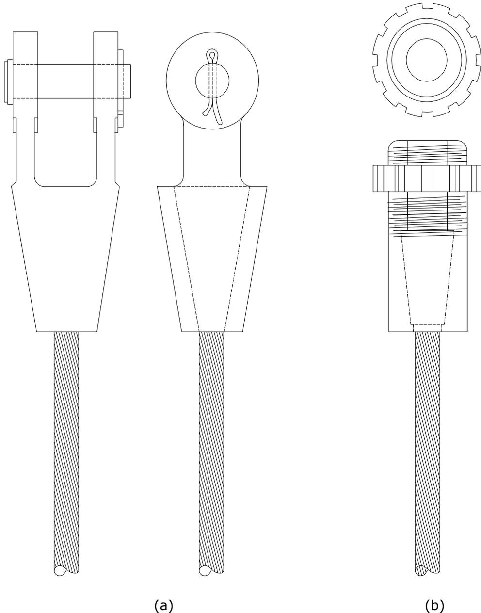
Figure 2.4 (a) Socket terminal with pin connector
