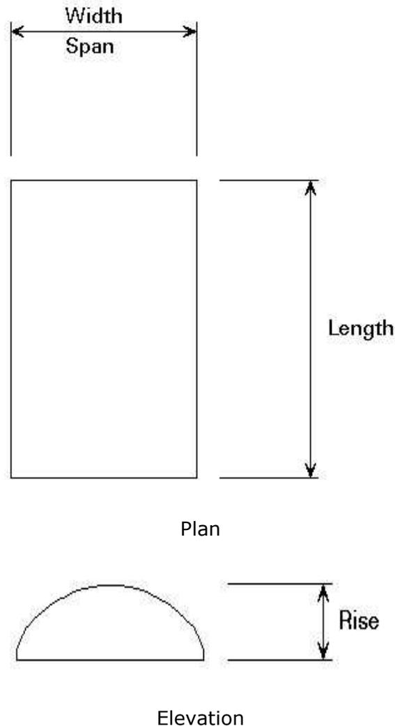
Figure 5.1 Braced barrel vault
