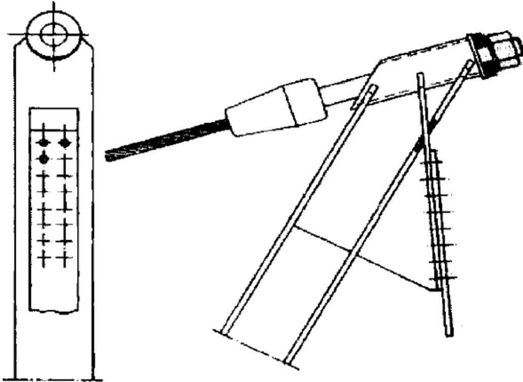
Figure 2.5 Attachment of cable with socket terminal to top of steel column
