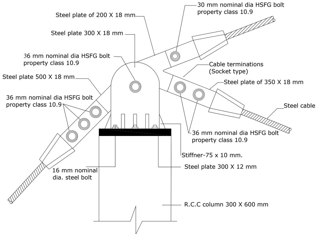
Figure 4.9 Elevation of cable-column connection (hinge connection)
