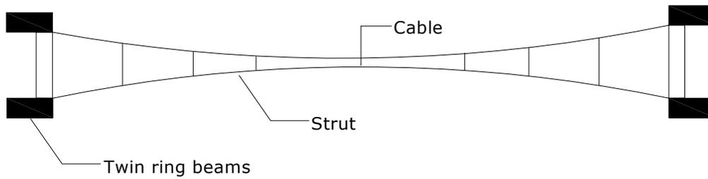
Figure-3.11 Double layer cable-concave shape for circular buildings
