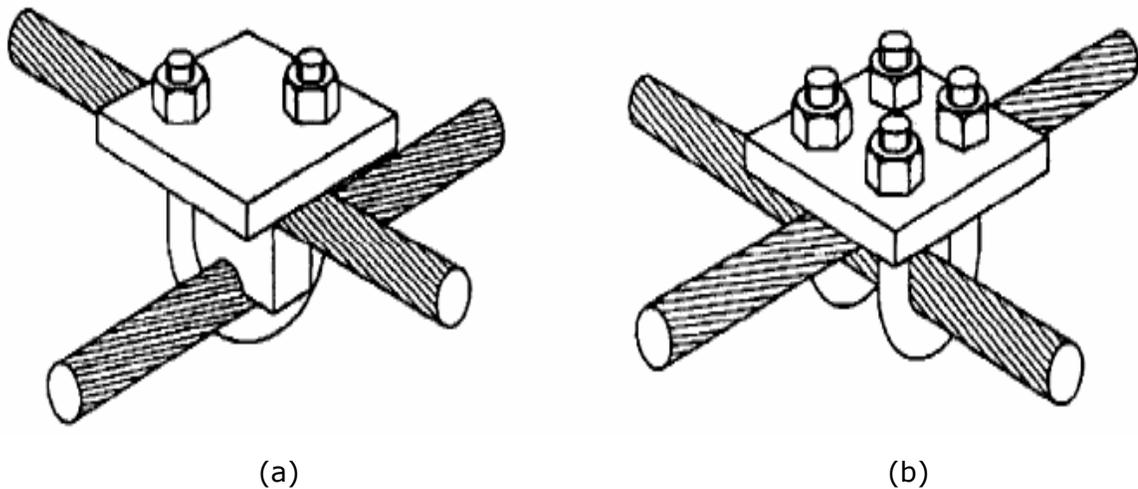
Figure 2.8 (a) Single u-bolt connection for cable net
