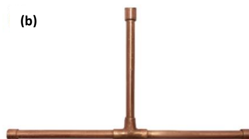
Fig. 3.2 Photographs of (a) Experimental setup (b) Multi-branch heat Pipe.
