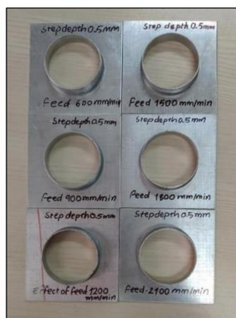
Figure 4.2 Flanges formed with different feed rate
