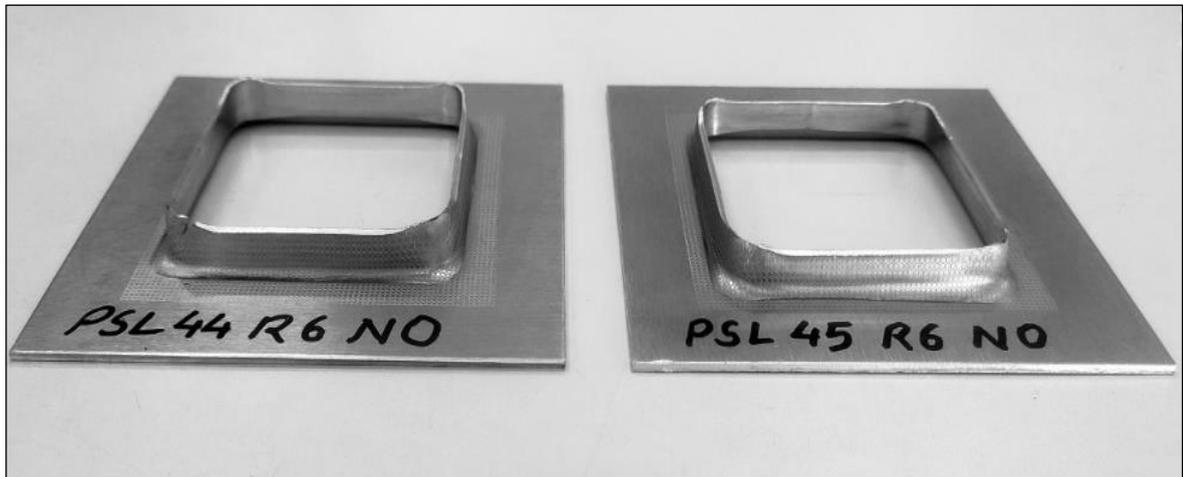
Figure 5.5 Failed and successfully formed flange by single-stage SPIHF
