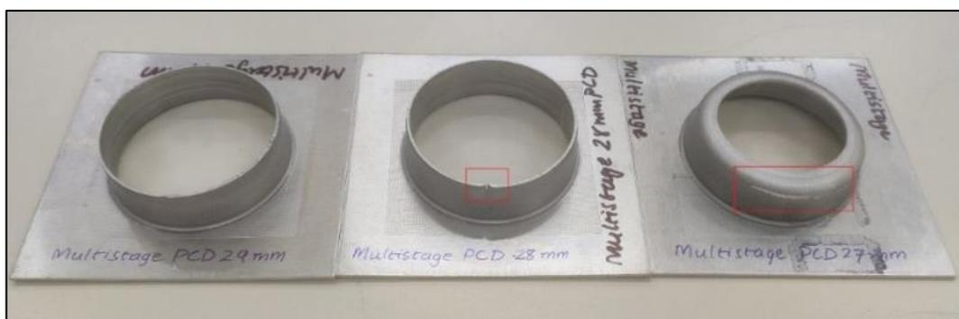
Figure 3.14 Flanges formed with the multistage strategy with pre-cut hole diameters 29mm, 28mm, and 27mm
