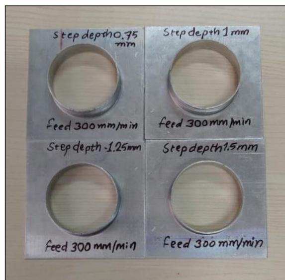
Figure 4.4 Flanges formed with different step depth
