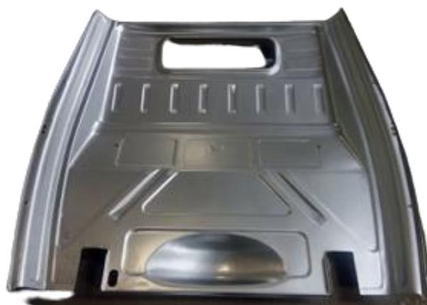
Figure 1.2 A rectangular flange on the assembly cabin rear wall of an automobile (courtesy- ASAL products, Pune, India)
