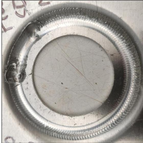
Figure 4.6 Damaged surface of AA5052-H32 sheet due to high values of process parameters
