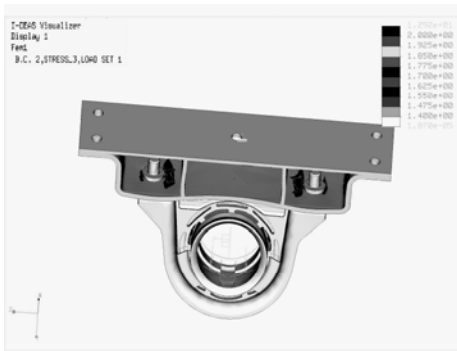
Fig. 2: Nastran Stress Plot, with max stress coming 251.6 N/mm 2
