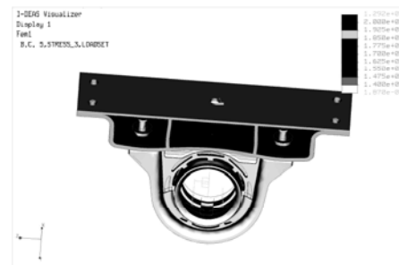
Fig. 4: Nastran Stress Plot, with max stress coming 129.2 N/mm 2
