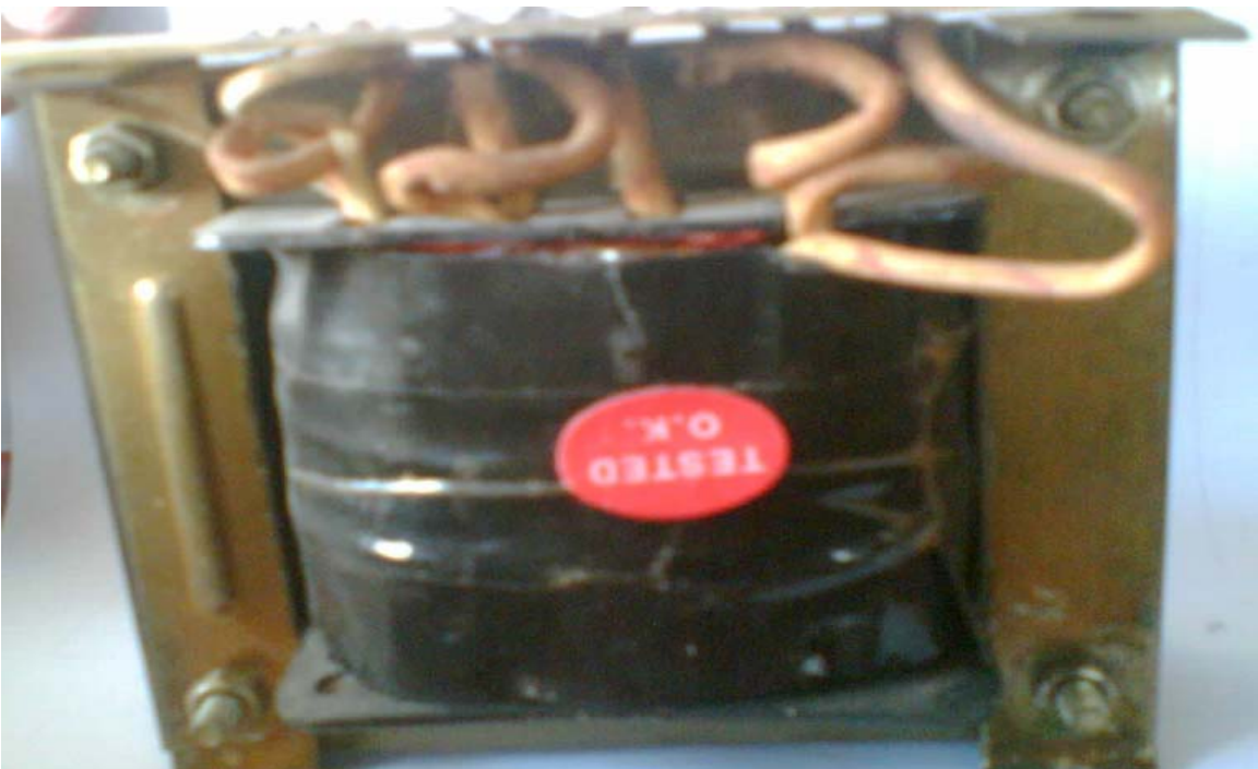
[11.10] Photograph of auto transformer:
