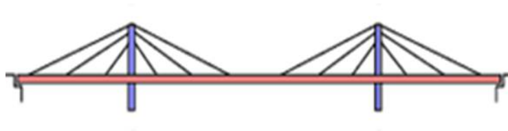
Figure 3.9: Typical arrangement of Semi Harp type arrangement
