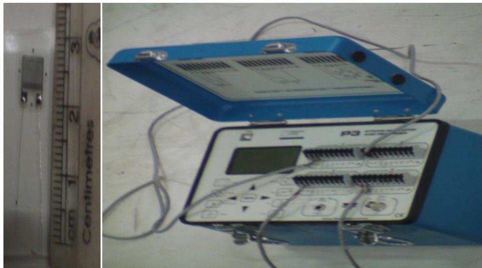
Figure 4.12: Strain Gauge of  $120\ \Omega$  with P3 Electrical strain gauge
