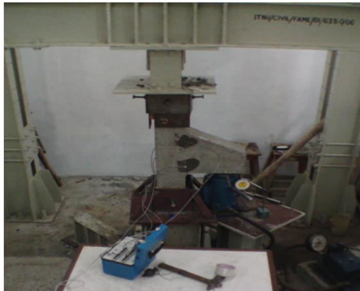
Figure 4.9: Vertical load applied to specimen
