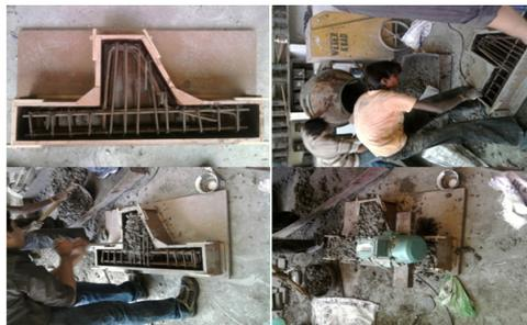
Figure 4.7: procedure for casting of specimen
