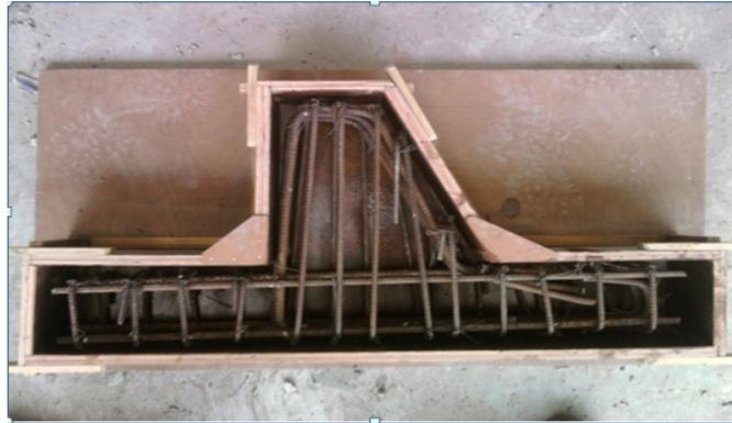
Figure 4.6: Reinforcement cage in mold
