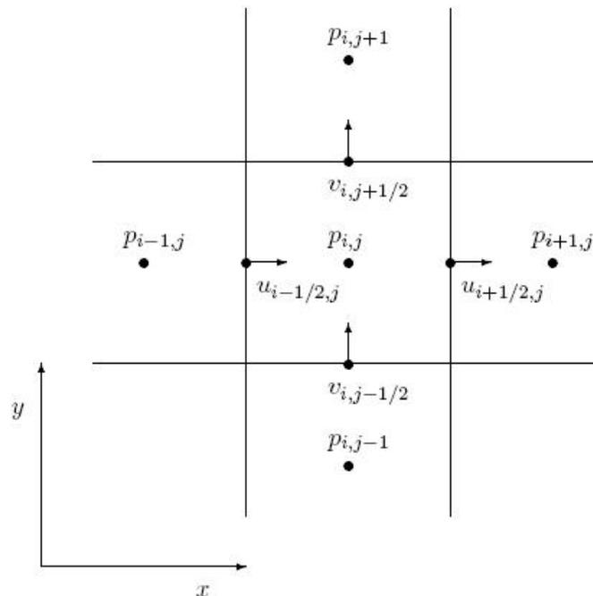
Figure 4.5: The two-dimensional grid
