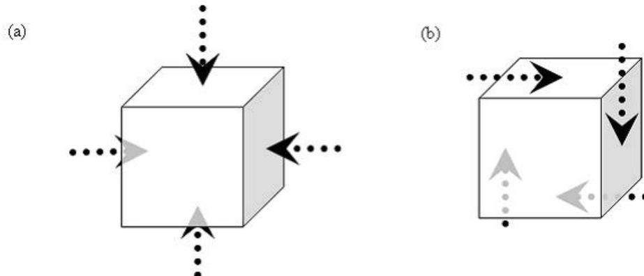
Figure 3.1: Components of stress: (a) normal (pressure) and (b) shear
