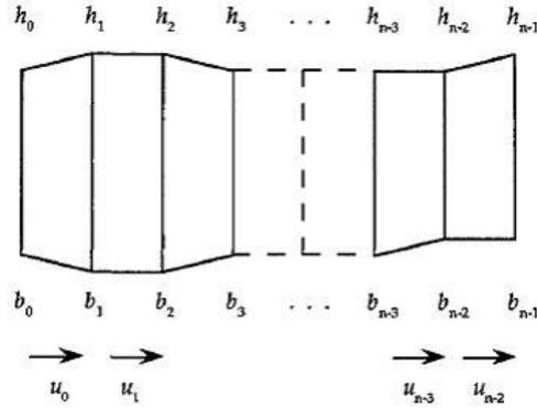
Figure 2.1: Discrete two-dimensional height-field representation of the water surface  $h$ , the ground bottom  $b$ , and the horizontal water velocity  $u$ .
