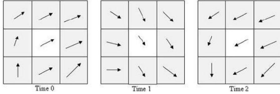
Figure 4.7: Eulerian acceleration: velocity at a fixed location changes over time.
