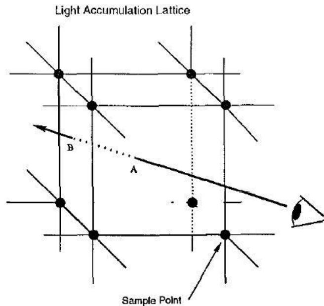
Figure 2.3: A viewing ray entering a Light Accumulation Lattice cell at point A and exiting at point B
