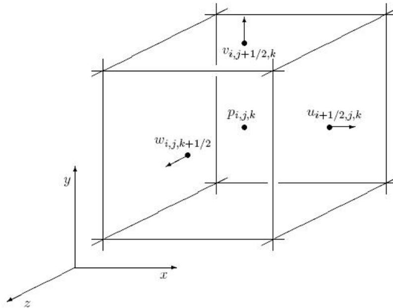
Figure 4.6: The Three-dimensional grid
