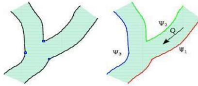
Figure 2.2: The stream function,  $\psi$  constant along all connected boundary.
