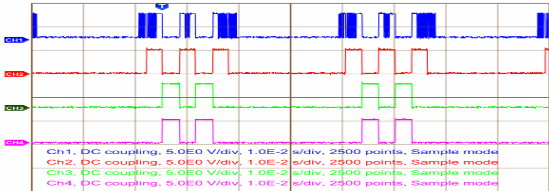
Fig. 7.2.4 : Signals Generated At Output of Logic Circuit @ 26 Hz (R-Phase)
