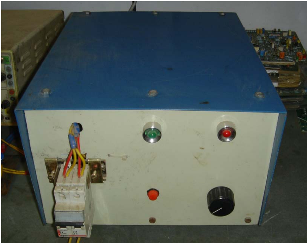
Fig. 9.6: Input side of the SCR based inverter welding machine
