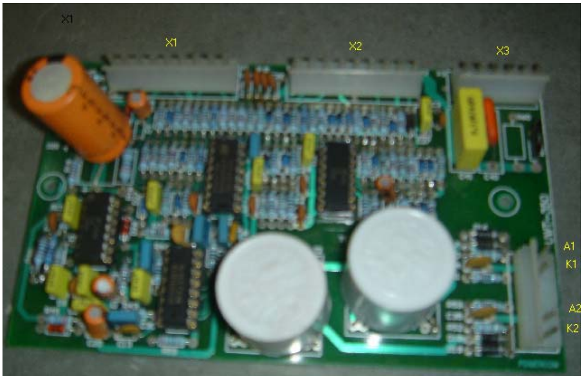
Fig. 9.3: Control card of SCR based inverter welding machine
