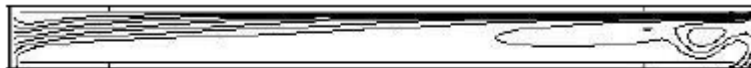
Figure 7: Streamline plot of the flow in the air gap with a height of 0.14m and an inclination angle of 25°.
