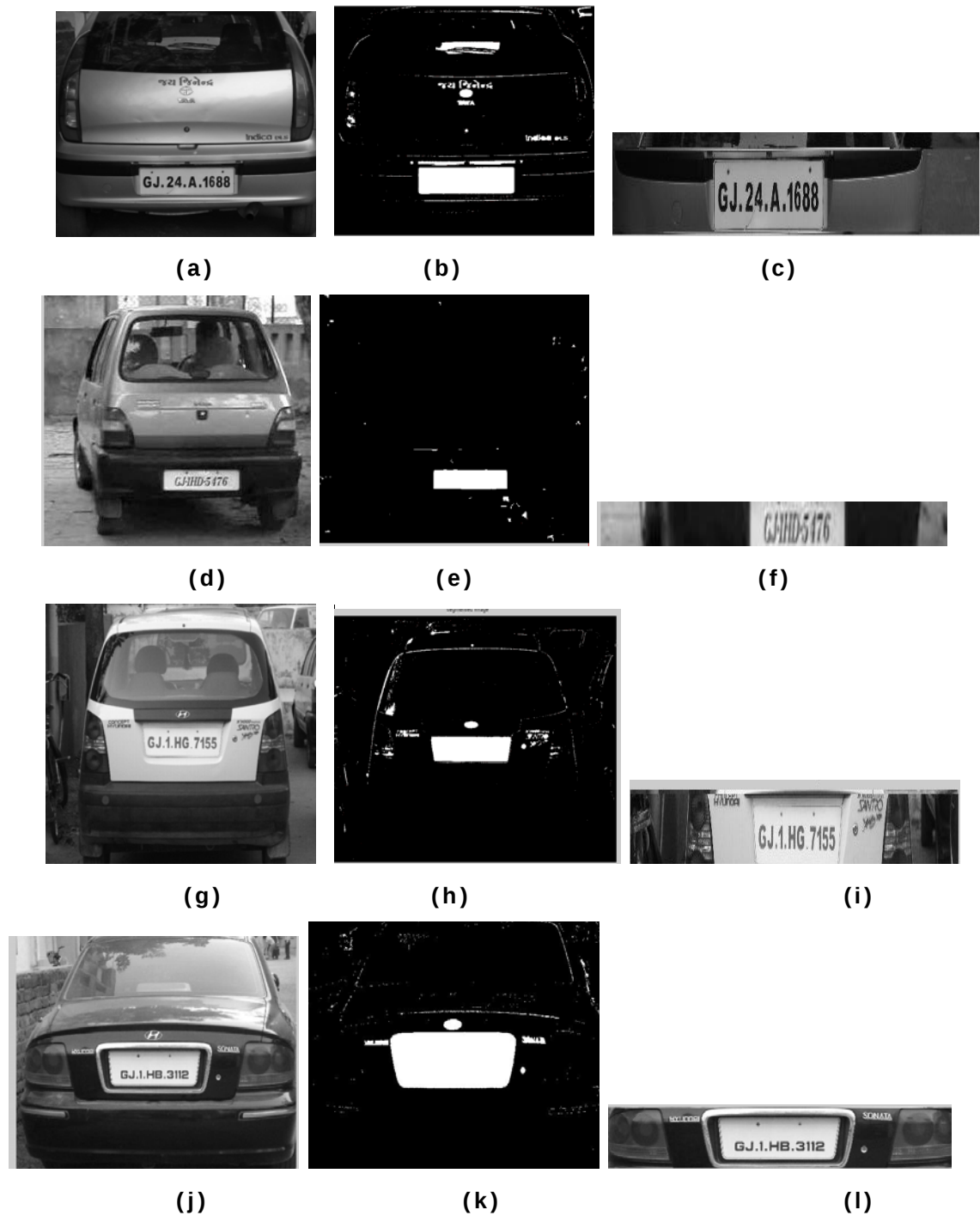
Figure-3.7 (a, d, g, j) – Original images (b, e, h, k) – results achieved with noise region, when applied Morphological technique (c, f, i, l) – Strip containing Number plate only
