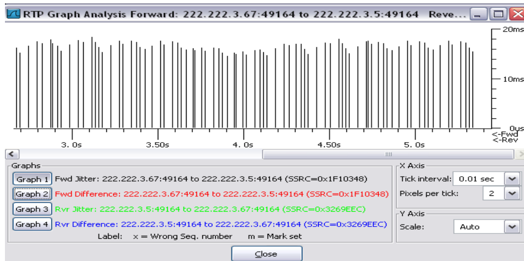
Figure 5.14 RTP graph for jitter analysis from 222.222.3.5 to 222.222.3.67
