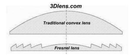
Below is a schematic cut-away diagram showing how a Fresnel lens is made.
