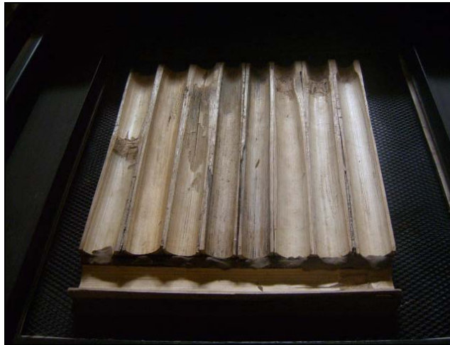
Figure 3 (c) Half split bamboo panel coated with glass fiber mat and GP resin
