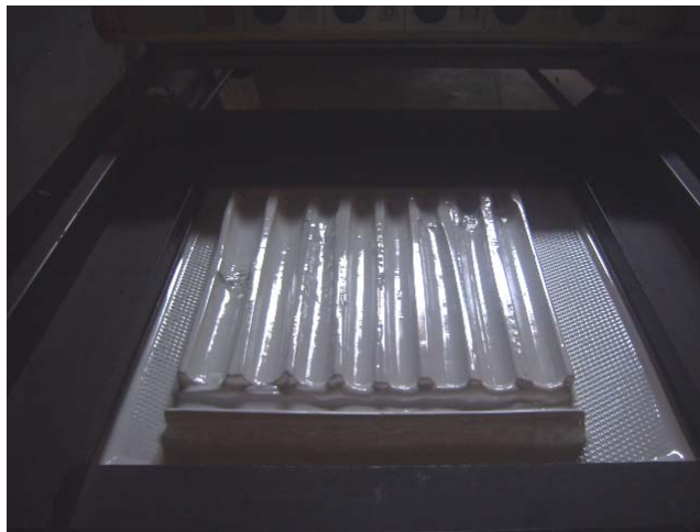
Figure 3 (c) Half split bamboo panel coated with glass fiber mat and GP resin
