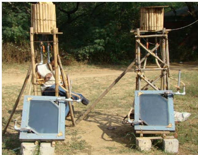
Figure 3 (f) Half split bamboo panel harvesting the solar energy
