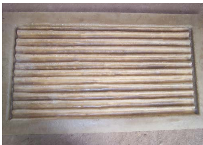
Figure 3 (f) Half split bamboo panel harvesting the solar energy
