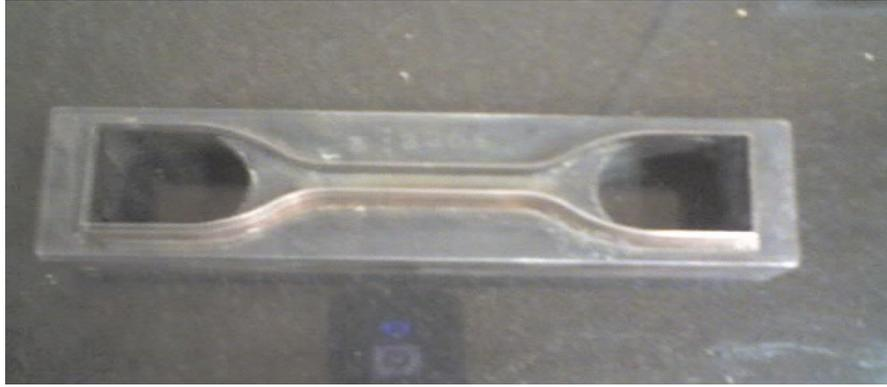
Fig 6.3 Die for the specimen type IV
