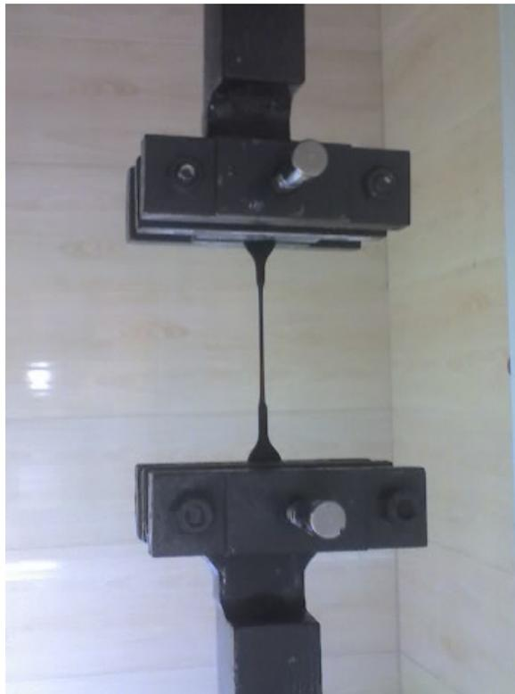
Fig 6.6 Elongation of specimen
