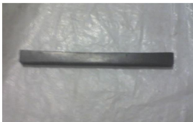
Fig 6.9 Specimen for flexural test
