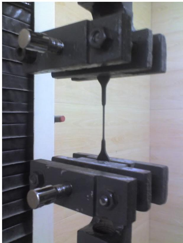
Fig 6.5 Placement of flat specimen for testing
