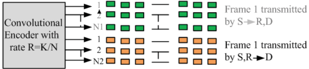
Figure 4.8: An example of the bit mapping for cooperation for a rate k/n convolutional code
