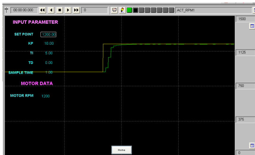
Figure 8.6: Speed control with PID tuning at speed set Pt.1200rpm
