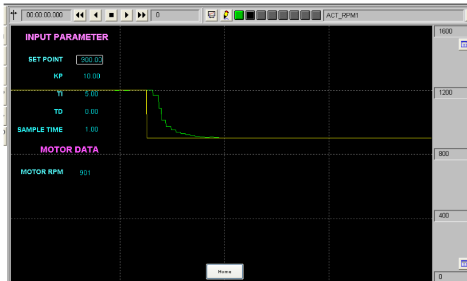
Figure 8.5: Speed control with PID tuning at speed set Pt.900rpm
