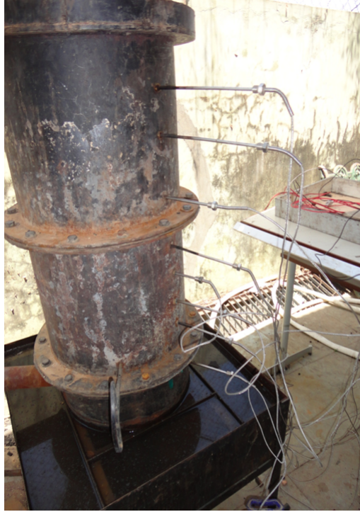
Figure 3.8: Thermocouple across the length of gasifier
