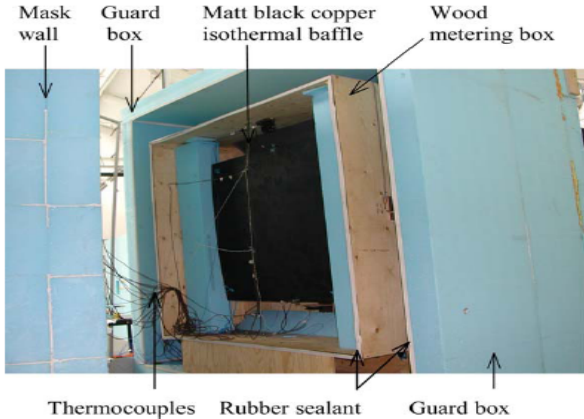
Figure 3.2: A photograph of guarded hot box by Fang et al
