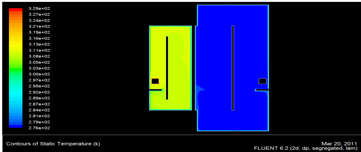
Figure 4.1: The temperature contours at a heat rate of 21 W for guarded hot box
