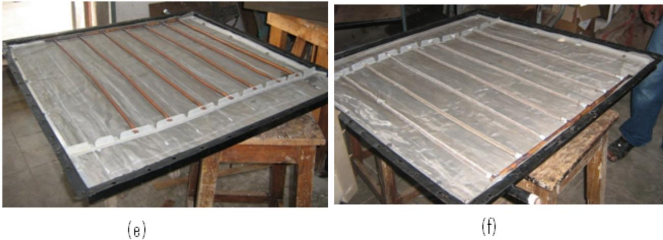
Figure 4.3: (e) Copper pipes connected with common header (f) Net provided on the pipes
