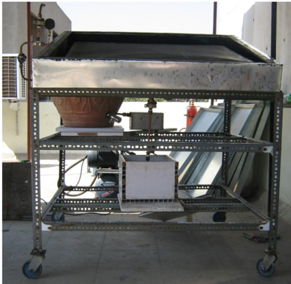
Figure 5.4: Photograph of solar adsorption chiller
