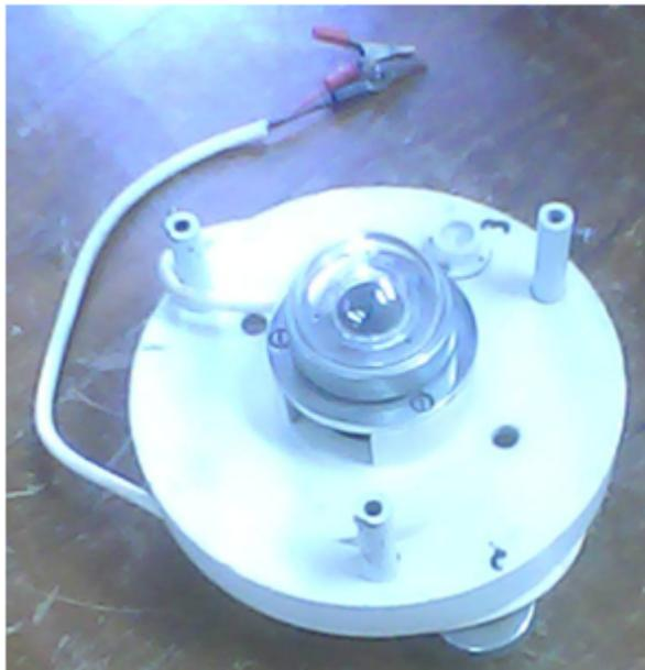
Figure 3.2: Pyranometer
