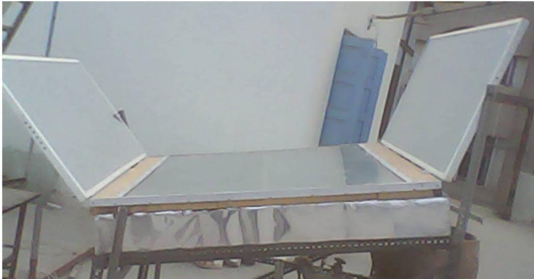
Figure 5.1: Collector with reflector
