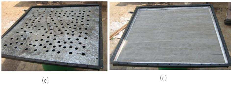
Figure 4.2: (c) Galvanized iron sheet with number of holes (d) Metallic mesh
