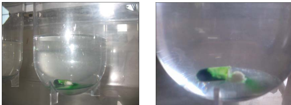
Figure : 4.28 Determination of lag time using colored granules
