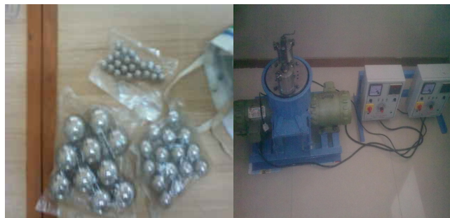
Fig. 2: Grinding Balls and High Energy Ball Mill (Planetary ball mill)
