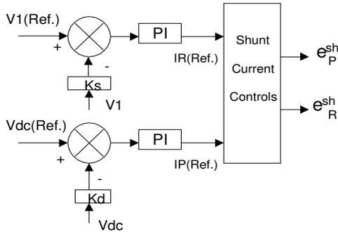
Figure (4): STATCOM current controller
