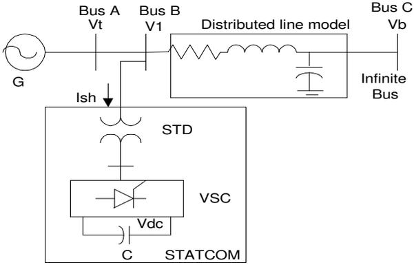
Figure (1): System with STATCOM at sending end of Line
