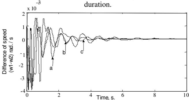
Figure (10): Response of the short scale multi-machine system with PI based STATCOM during three phase short circuit at bus 7 a. located at 'a' b. located at 'b' c. located at 'c'
