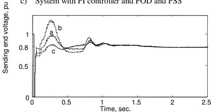
Figure (9): Three Phase fault at Sending end with 50ms duration.
