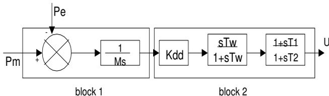
Figure (5): Transfer function block diagram of the POD
