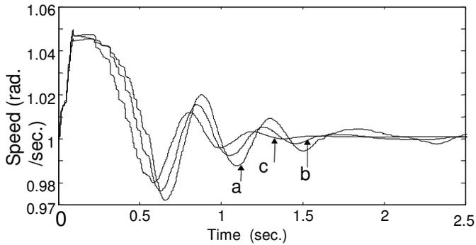
Figure (8): Response of the SMIB system with PI based STATCOM
