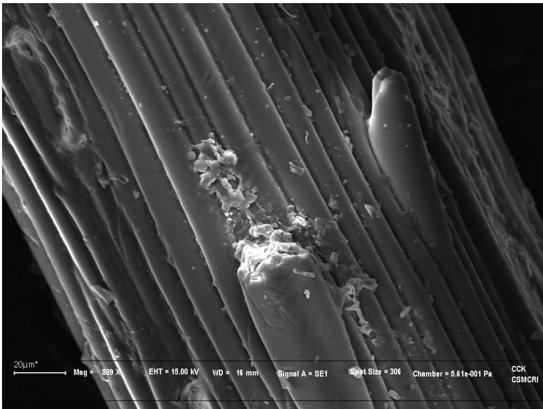
Figure 31 SEM image of untreated Wheat straw
