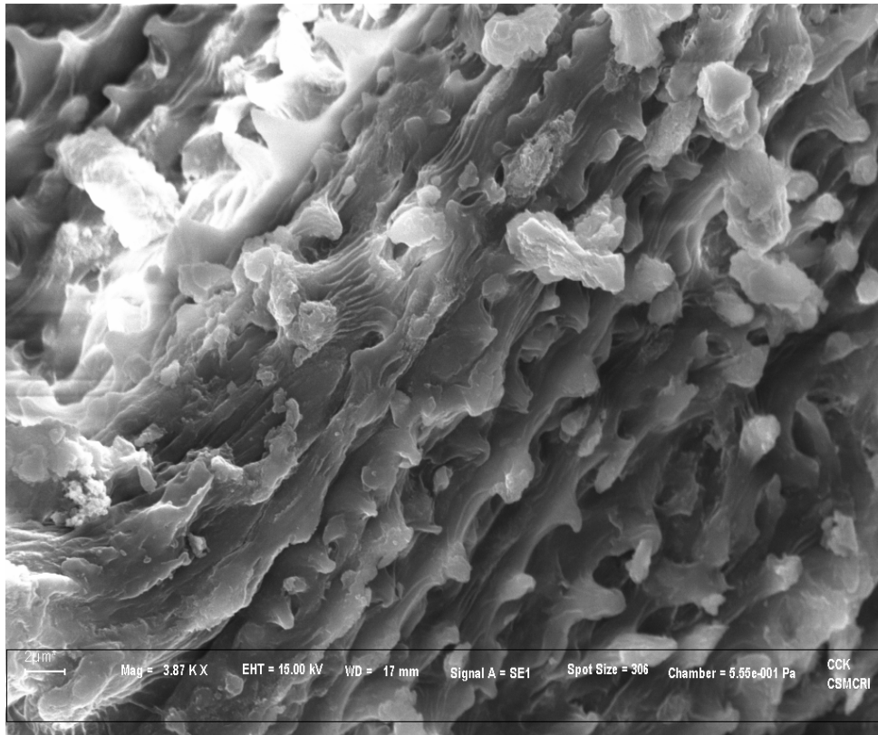
Figure 32 SEM image of 10% NaOH treated Wheat straw
