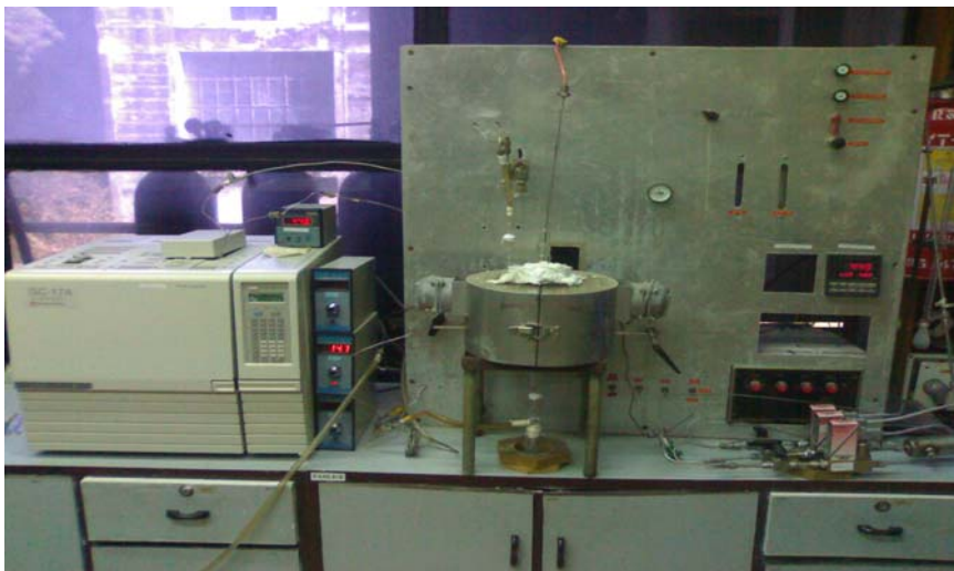
Fig. 4.1 Experimental setup for catalyst evaluation
