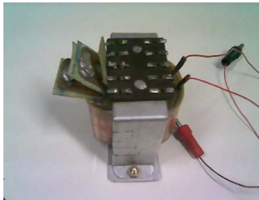
Figure 3.2: View of 'E' Core Transformer with Copper Strips
