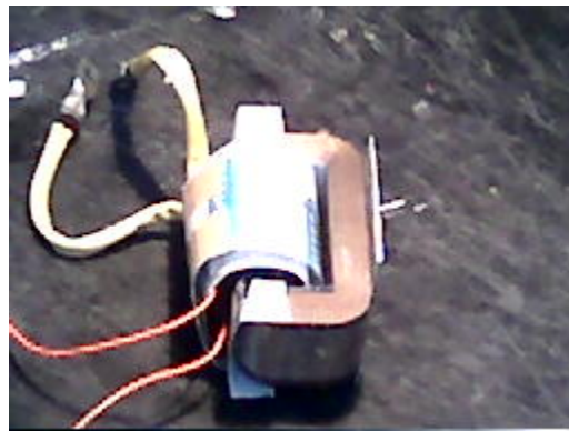
Figure 3.4: View of Transformer with ‘C’ Core
