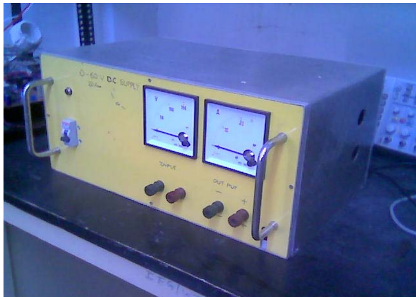
Figure 3.8: Complete View of 60 Volt Variable DC Supply
