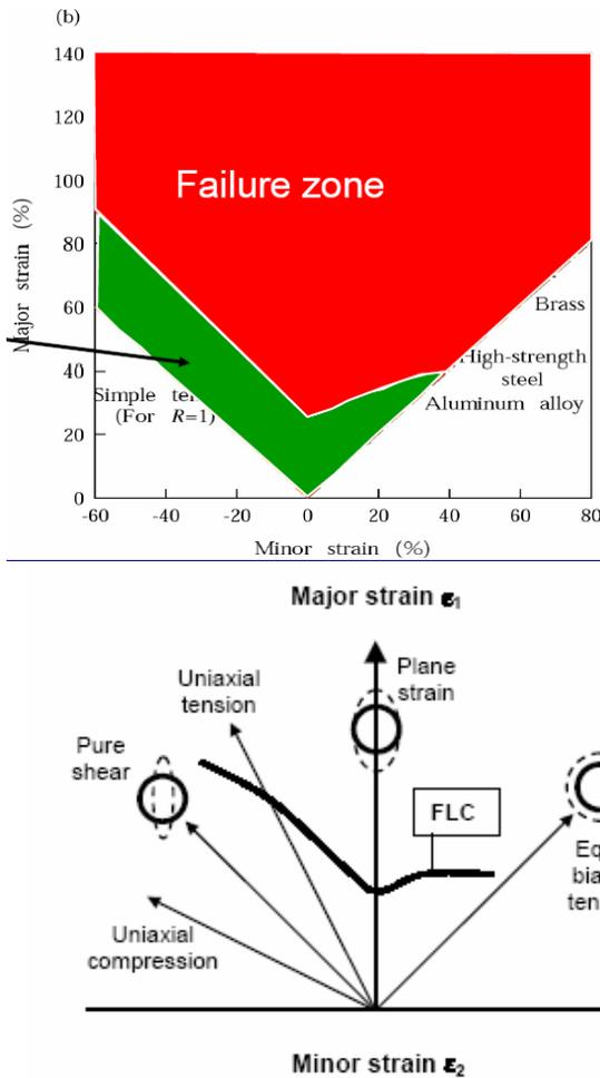
Fig. 1. Forming limit curve
