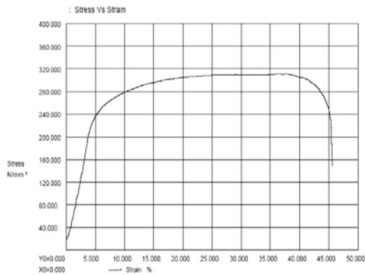
Fig 8. Stress Strain Curve by Tensile Test
