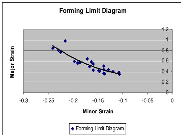
Fig 9. Forming Limit Diagram by tensile test
