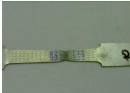
Fig 6. Deformed Specimen of Tensile Test
