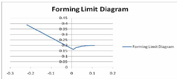
Fig 4. FLD based on Swift-Hill Model
