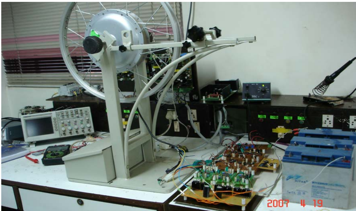
Fig 6.12 Complete experimental set-up of PWM controlled PMSLDC Motor Drive for Electric Vehicle
