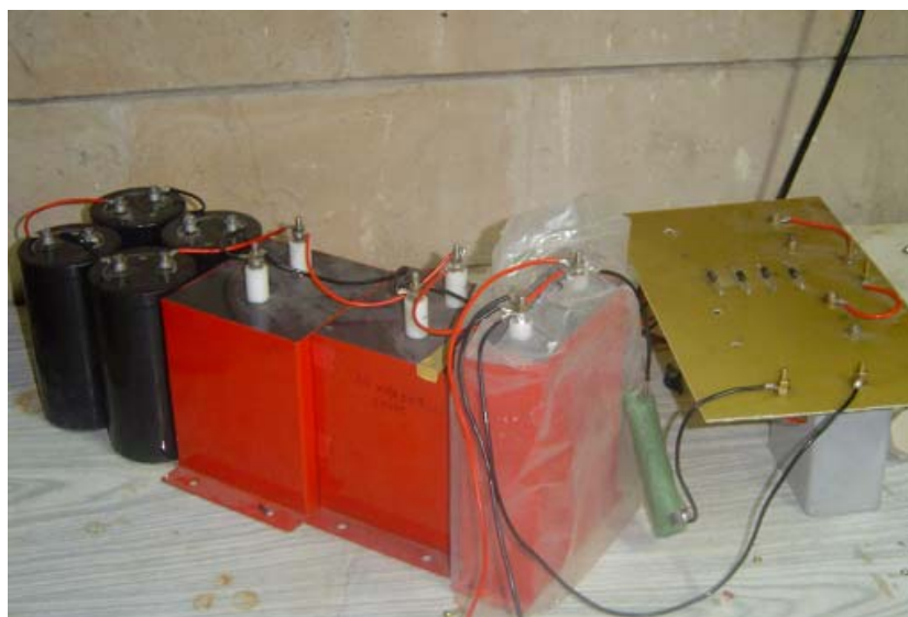
Figure (6.9): visual image of the capacitor bank used in the circuit
