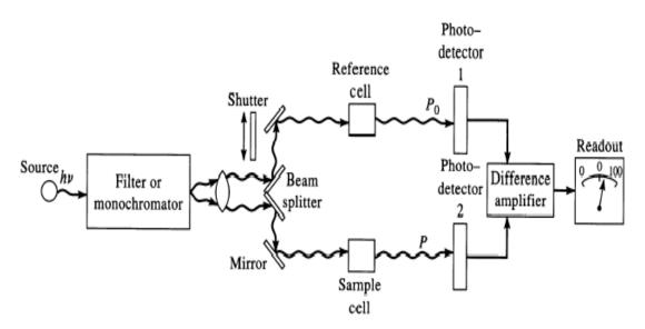
Fig 1.1: Double Beam UV Spectrophotometer
