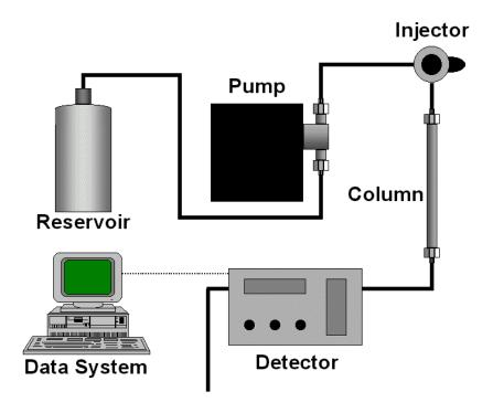
Fig. 1.4: A Flow Scheme of HPLC
