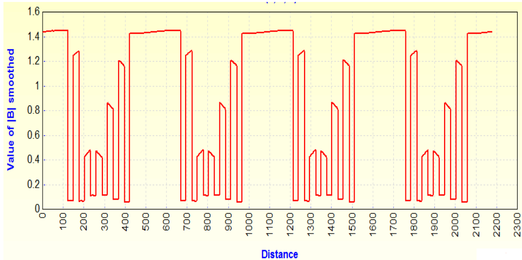
Figure 6.11: Graphical Representation of Flux Density at Rotor Teeth
