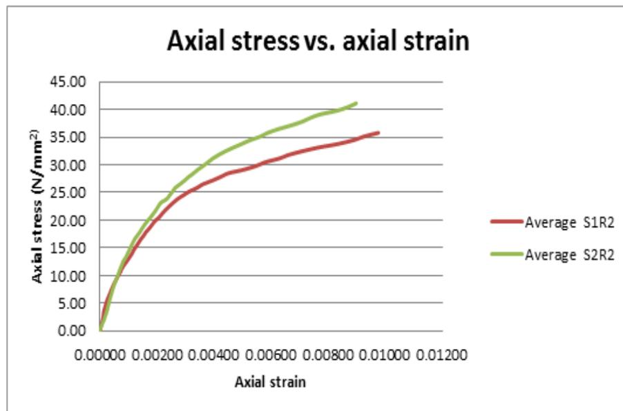
Figure 5.16: R2 corner radius with one layer and two layers
