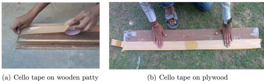
Figure 4.8: Application of cello tape on the surface of wooden patty and plywood
