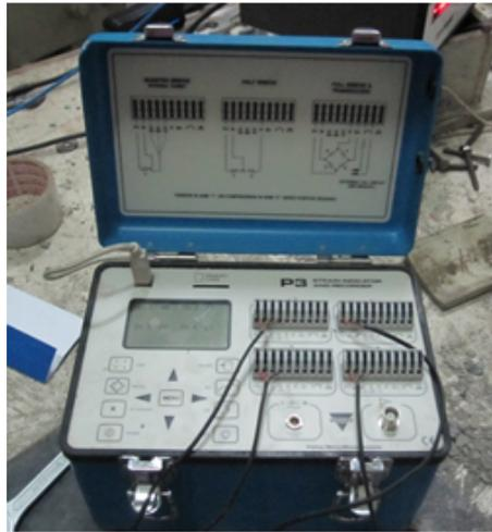
Figure 4.21: P3 strain indicator and recorder
