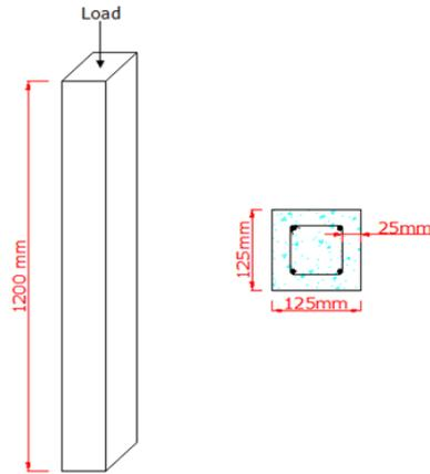
Figure 3.1: RC column with cross section
