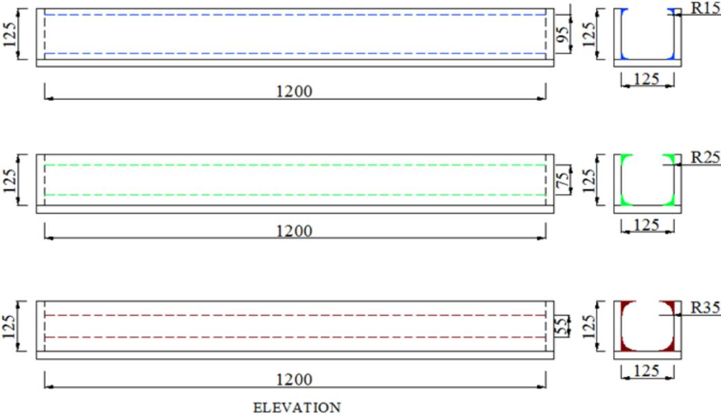
Figure 4.6: Schematic view of formwork for columns with corner radius 15mm, 25mm and 35mm
