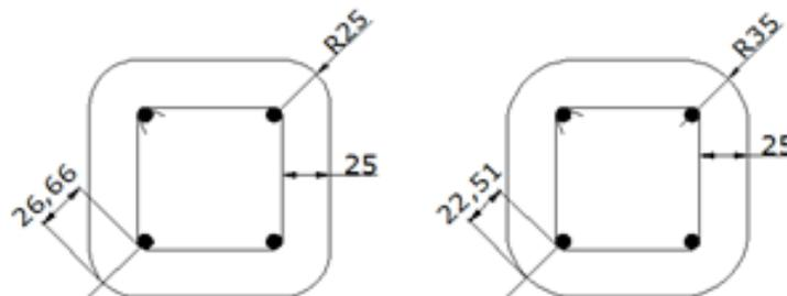
Figure 5.7: Variation in clear cover with different corner radius
