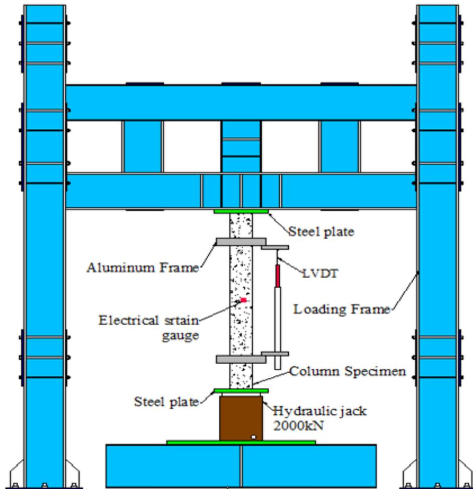
Figure 4.18: Schematic view of test setup for axial load
