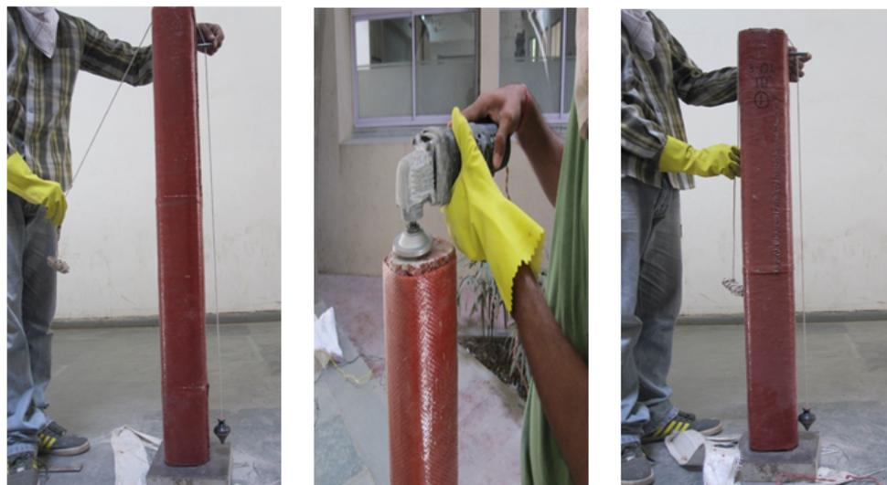
(a) Before levelling of column (b) Grinding on the top and bottom (c) After grinding of base
