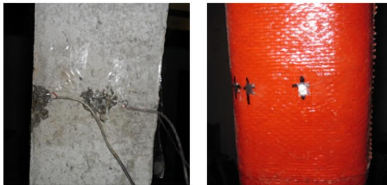
(c) Strain gauges onto surface of concrete (d) Strain gauges onto surface of GFRP
