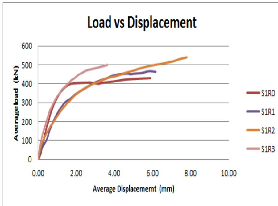
Figure 5.12: Single layer wrapped specimen with different corner radii
