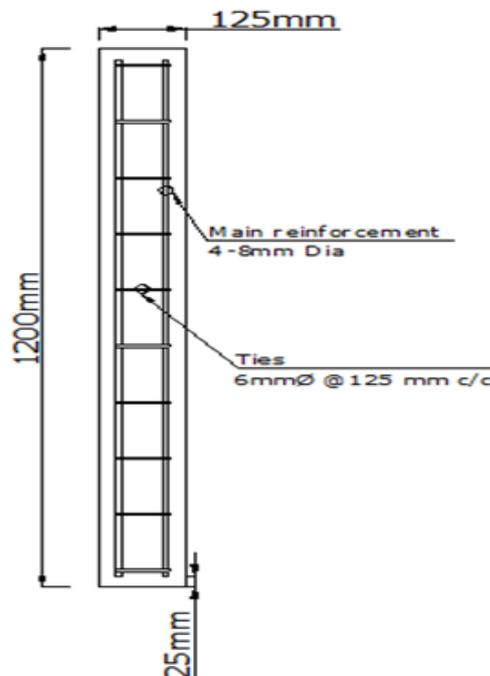
Figure 3.2: Reinforcement details of control RC column
