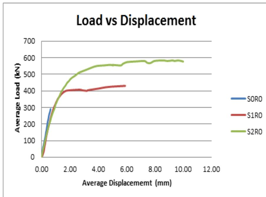
Figure 5.8: R0 corner radius specimens with single and double layers
