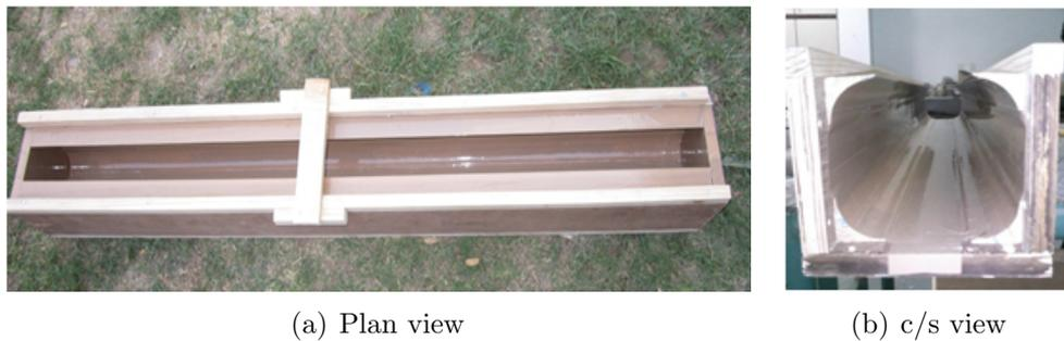
Figure 4.7: Completed formwork with corner radius patty
