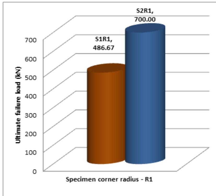
Figure 5.2: R1 columns with corner radius
