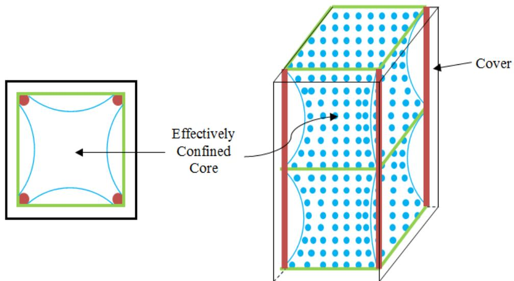
Figure 1.1: Development of confined core in column
