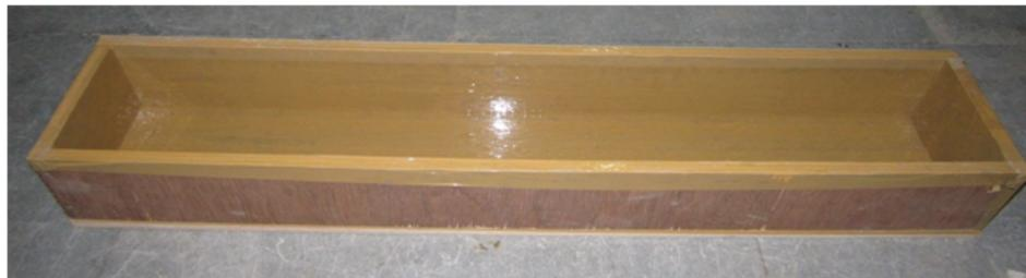
Figure 4.4: Completed formwork with sharp edges
