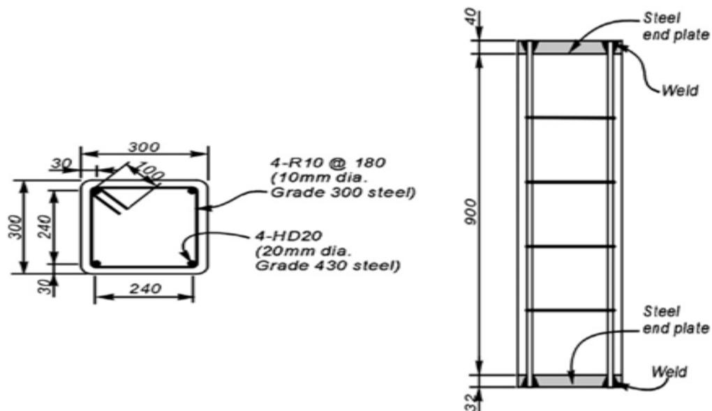
Figure 2.6: Reinforcing details of Square column
