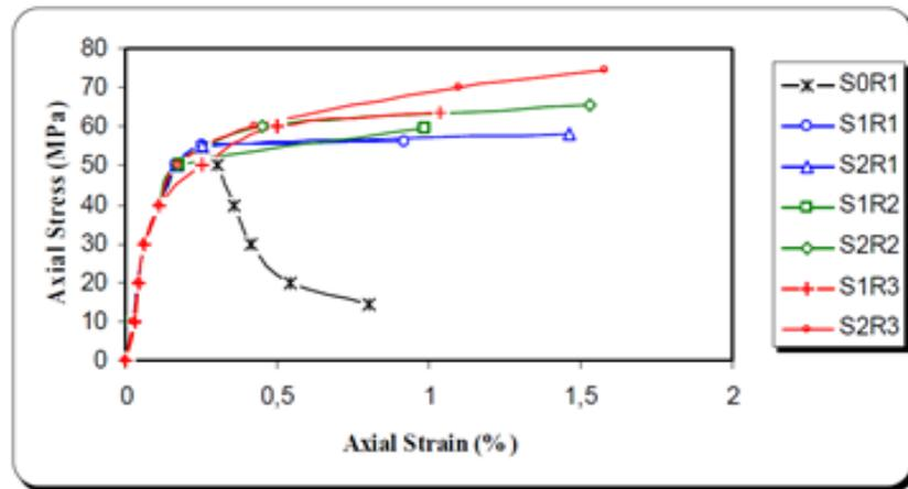
Figure 2.9: Stress-strain curves
