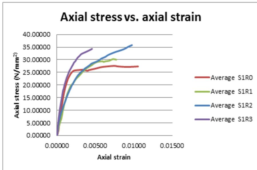
Figure 5.18: Single layer with different corner radius
