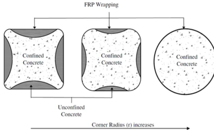
Figure 2.3: Effect of corner radius on confined concrete in square and cylindrical columns
