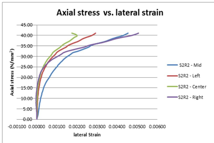
Figure 5.20: Strain at mid, left, Center and Right of S2R2
