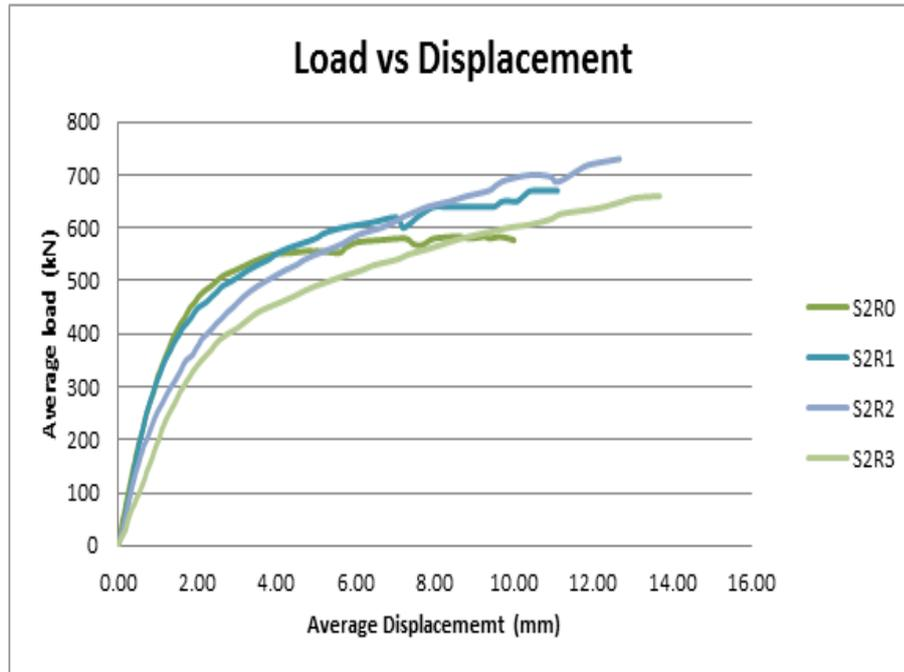
Figure 5.13: Double layer wrapped specimen with different corner radii
