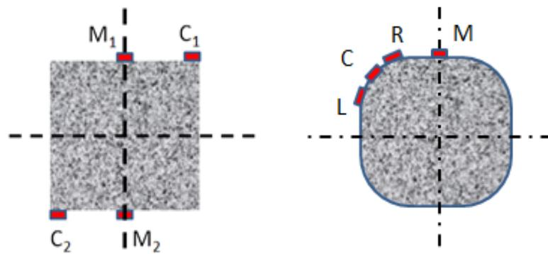
(a) Location of strain gauges on sharp edges (b) Location of strain gauges on corner radius
