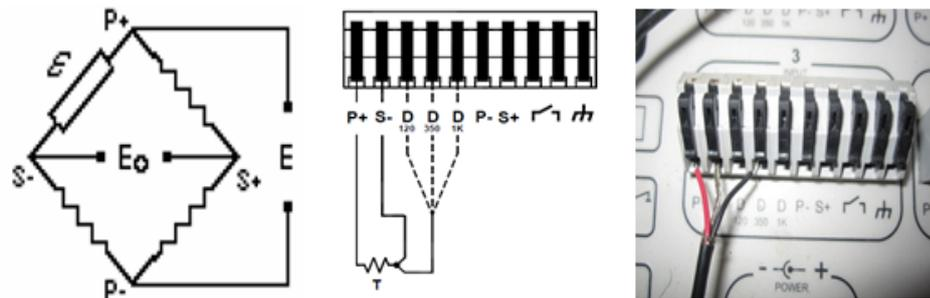
(a) Single active gauge in uniaxial tension or compression
