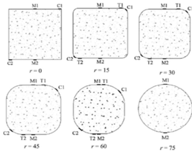
Figure 2.8: Strain gauge arrangements
