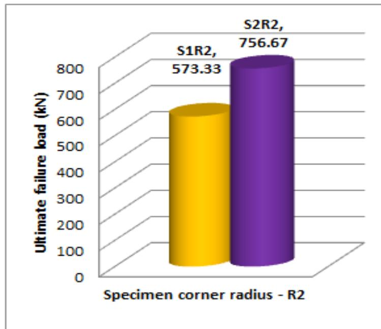
Figure 5.3: R2 columns with corner radius
