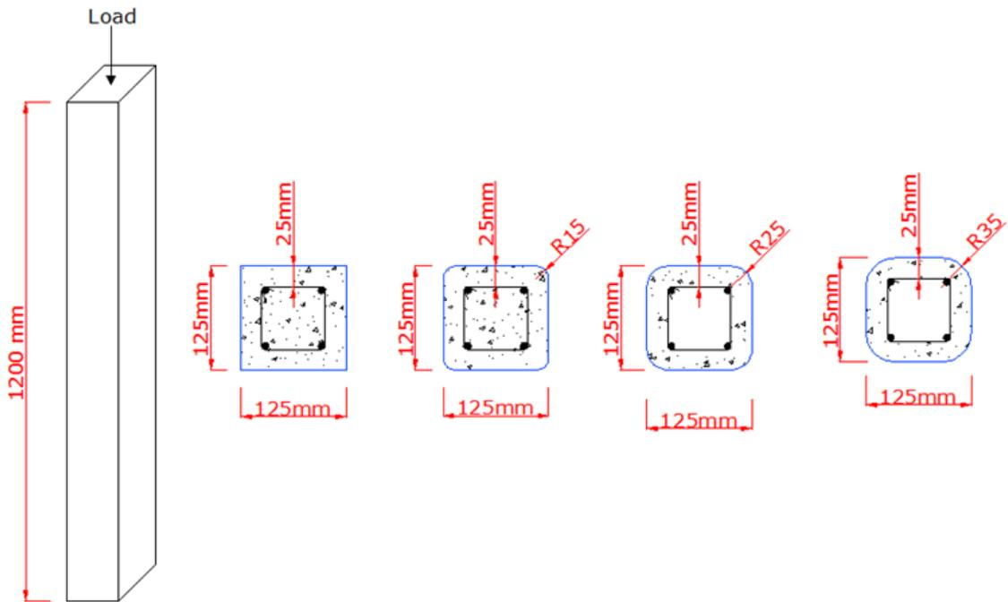
Figure 3.3: RC column with different corner radii
