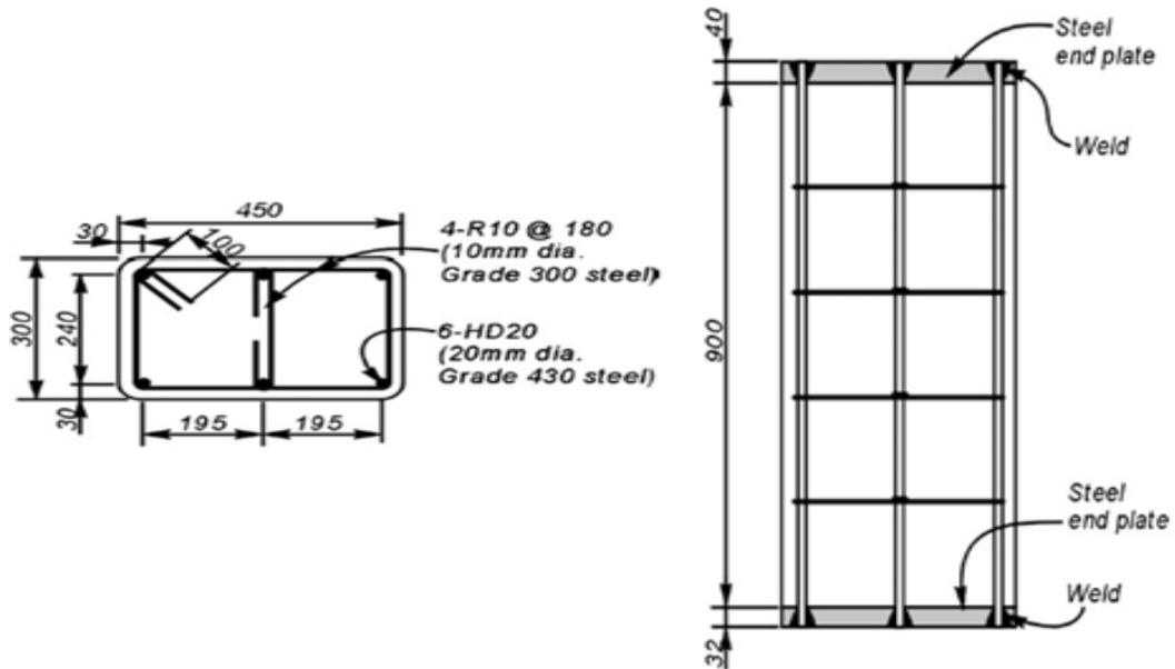
Figure 2.7: Reinforcing details of Rectangular column
