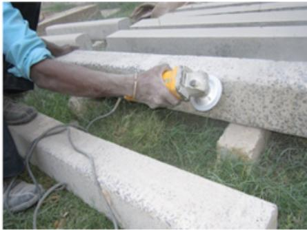
Figure 4.12: Grinding of column specimen
