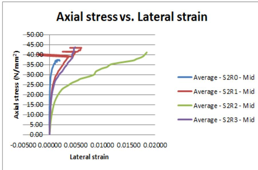
Figure 5.22: Double layer with different corner radius
