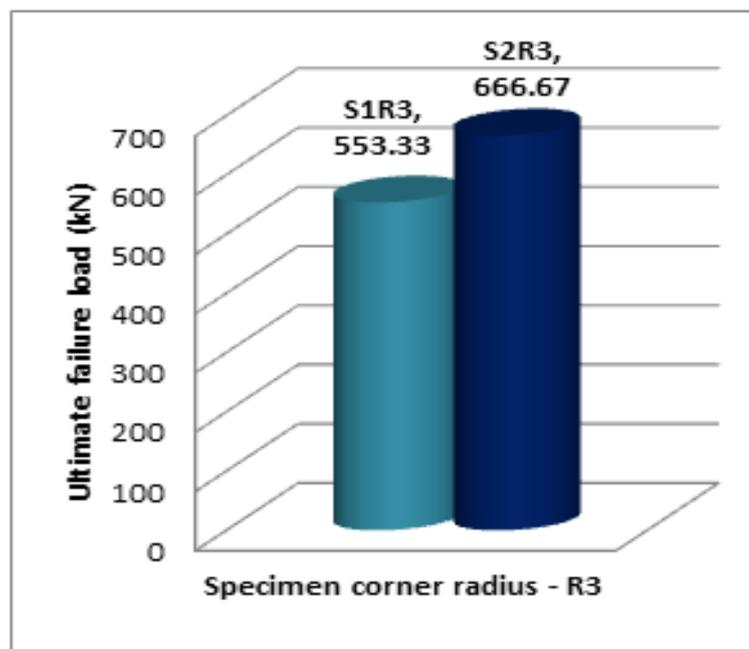
Figure 5.4: R3 columns with corner radius
