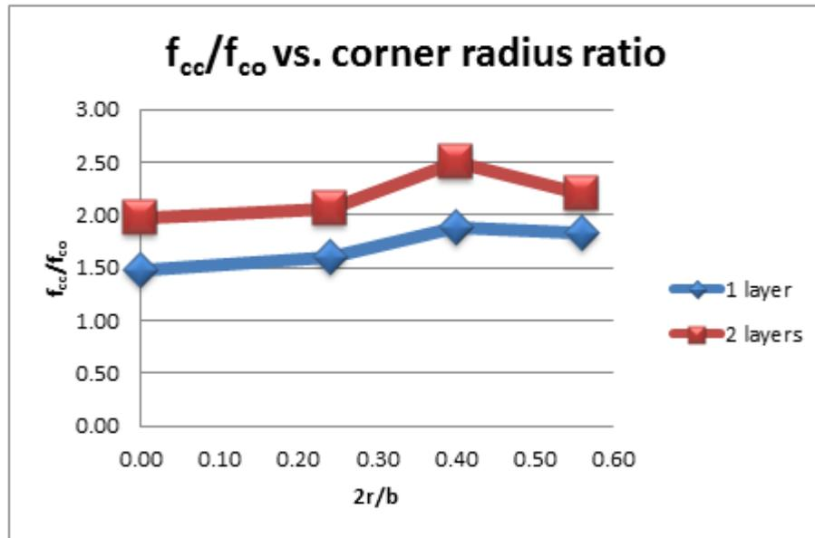
Figure 5.23: Strength gain of confined concrete vs. corner radius ratio
