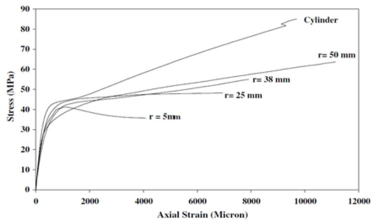
Figure 2.2: Effect of corner radius on confined square columns
