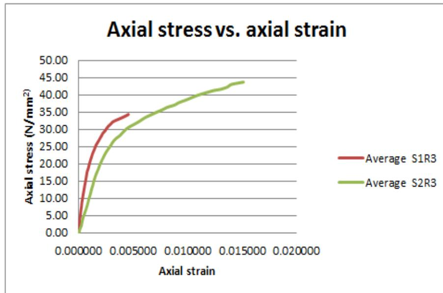
Figure 5.17: R3 corner radius with one layer and two layers
