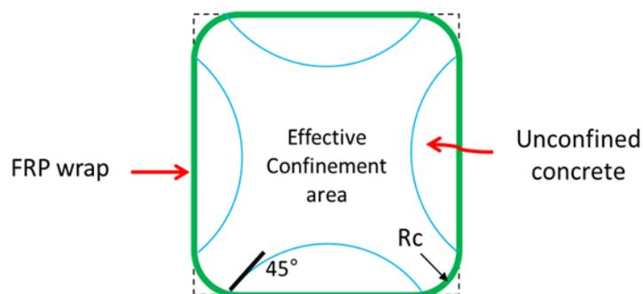
Figure 1.2: Effectively confined concrete in a square column
