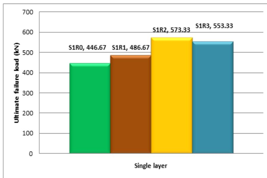
Figure 5.5: Column wrapped with single GFRP layer
