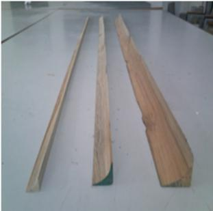
Figure 4.5: Different types of corner wooden patty
