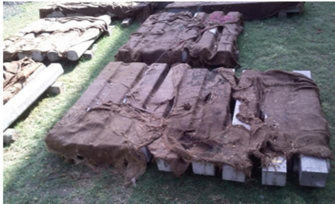
Figure 4.11: Curing period of specimens
