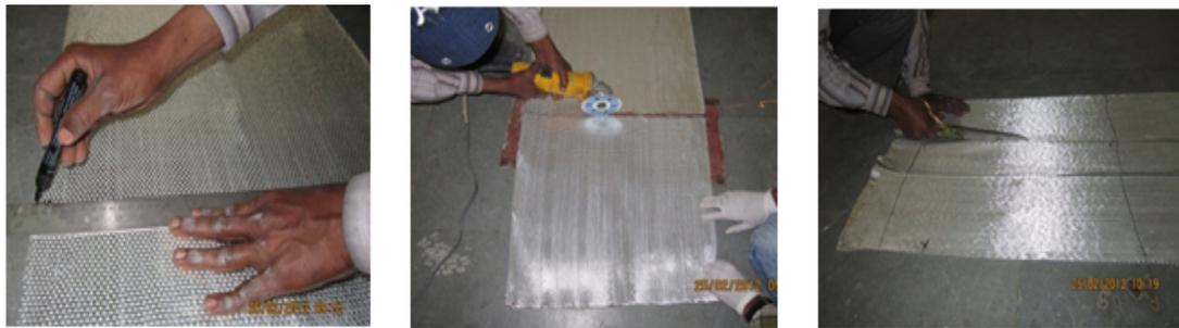
(a) Measuring of GFRP sheet (b) Cutting of GFRP sheet in transvers direction (c) Cutting of GFRP sheet in longitudinal direction
