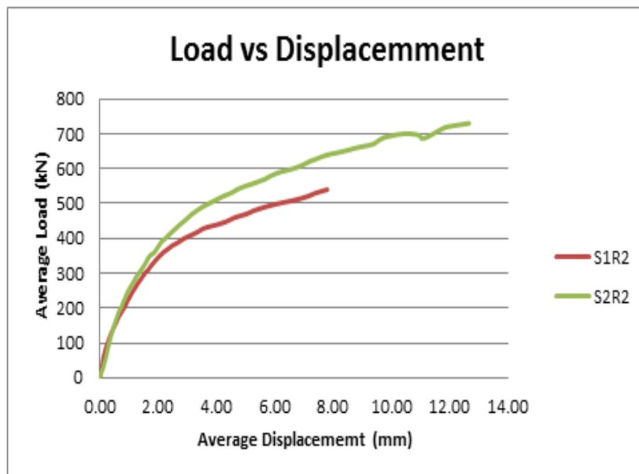
Figure 5.10: R2 corner radius specimen with single layer and double layers
