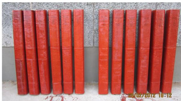
(e) After application of GFRP sheet and saturant
