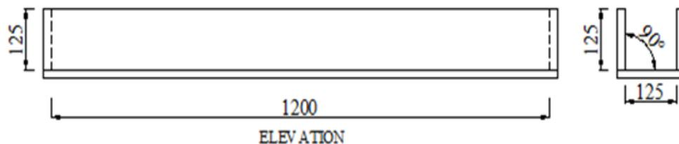
Figure 4.3: Schematic view of formwork with sharp edges
