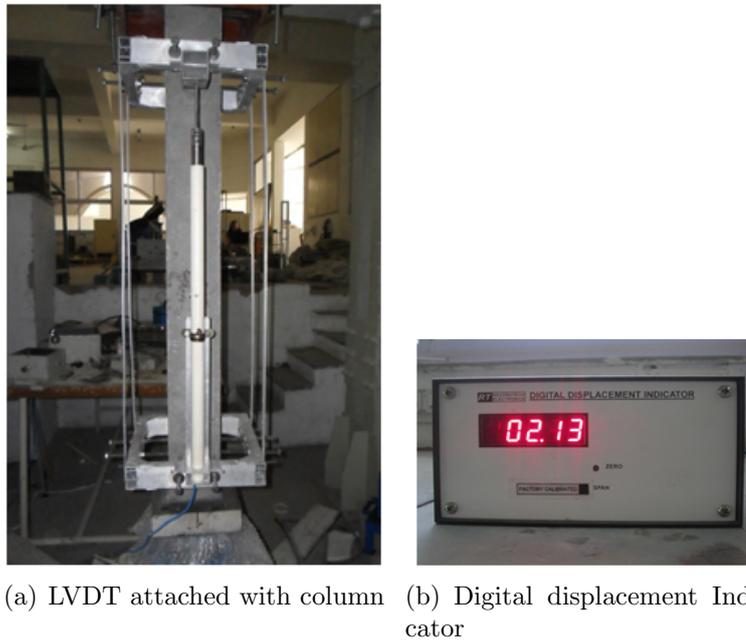
Figure 4.20: LVDT with aluminium setup
