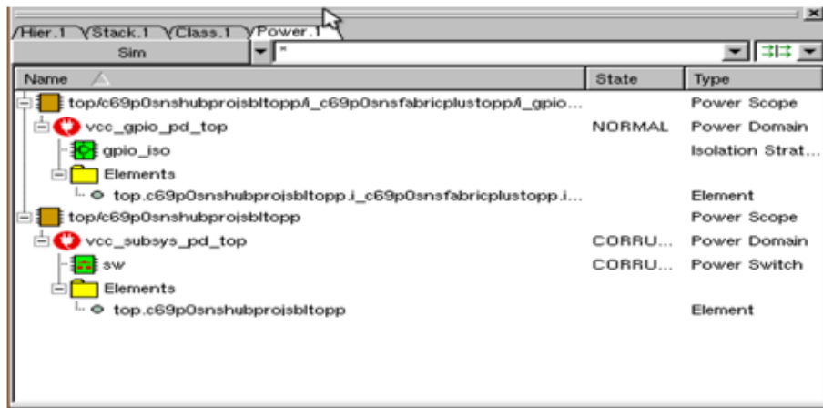
Figure 11.4: Power Switch And Isolation Cell
