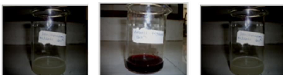
Figure 3.10: Lanthanum Nitrate / Cobalt Nitrate /  $\text{Na}_2\text{CO}_3$  Mix with 15 ml distilled water
