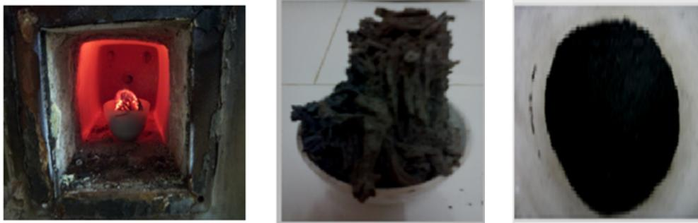
Figure 3.7: After Calcination in Muffle Furnace at 800 °C
