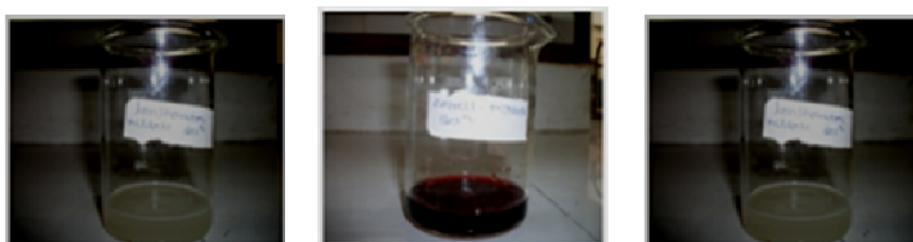
Figure 3.4: Lanthanum Nitrate / Cobalt Nitrate / Citric Acid Mix with 15 ml distilled water
