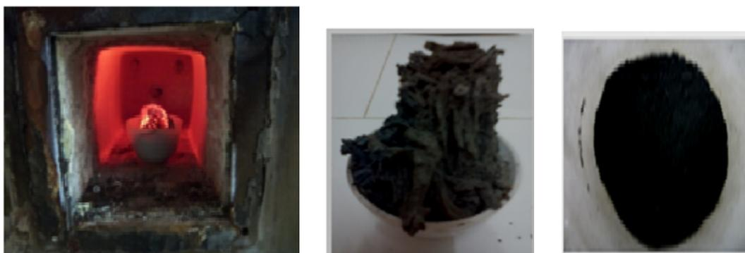
Figure 3.13: Calcination at 750 °C in Muffle Furnace
